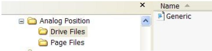
The Drive File directory contains a list of drive files for this application. The Drive file contains the upload and down load parameter values as well as parameter names, Modbus addresses, scaling, default values. The parameter values in the Drive File are the data actually downloaded / uploaded from the drive. Drive file is named Generic in above example.
