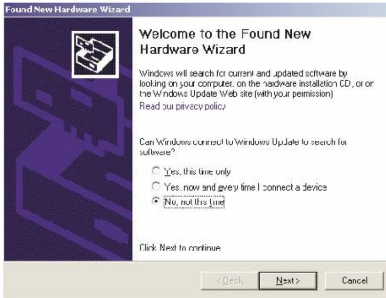
1. Plug the TTUSB485 into an available USB port on your computer or connected hub. The screen above appears, telling you that there is a new device plugged into the USB bus. Click on *No, not this time*, then the **Next>** button.
