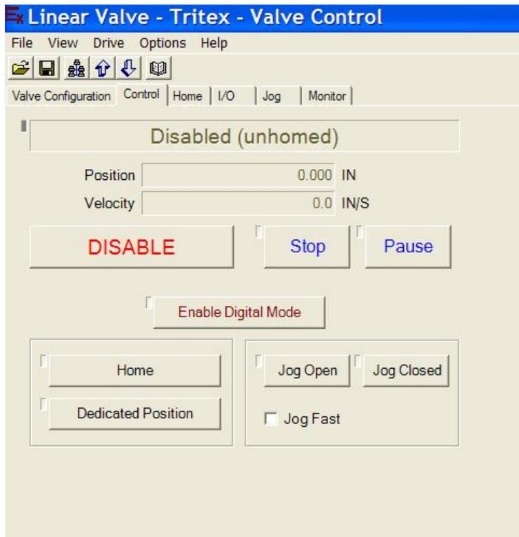
The Control page can be used for starting and stopping motion directly from the screen.
