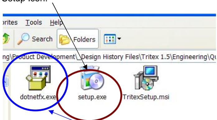
Expert software version 1.4.2.0 and later require Microsoft .NET Framework version 2.0 to be installed on the PC. If this version of .NET Framework is not on the PC a Microsoft message will be displayed suggesting you go to [Microsoft.com](http://Microsoft.com) to download it. This is not necessary as a distributable version of .NET Framework 2.0 has been included on the CD, it can be installed by clicking on the donetfx.exe file.
