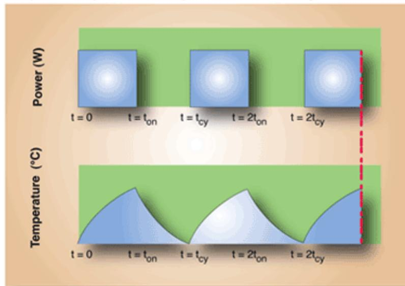
In summary, a temperature sensor won't always protect the motor's winding from overheating or even burning up.
