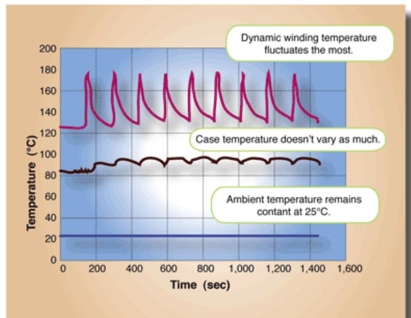
Next, our motor is pulsed with 3× peak current pulses: It is on for two seconds, and then off for 132, and cycled nine times. The measured 1.492% duty cycle agrees well with the 1.5% value calculated by the four-parameter model. During each two-second on period, measured winding temperature rises from 130° to 180° C; it takes the full 132 seconds for the winding to cool back to 140° C. Meanwhile, case temperature fluctuates slightly around 100° C — also predicted by the four-parameter model.
