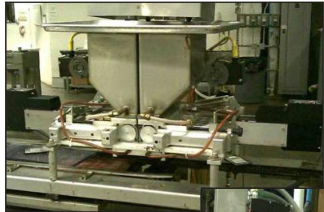
*Above: Chocolate dispensing machine with two Exlar T2M actuators*
