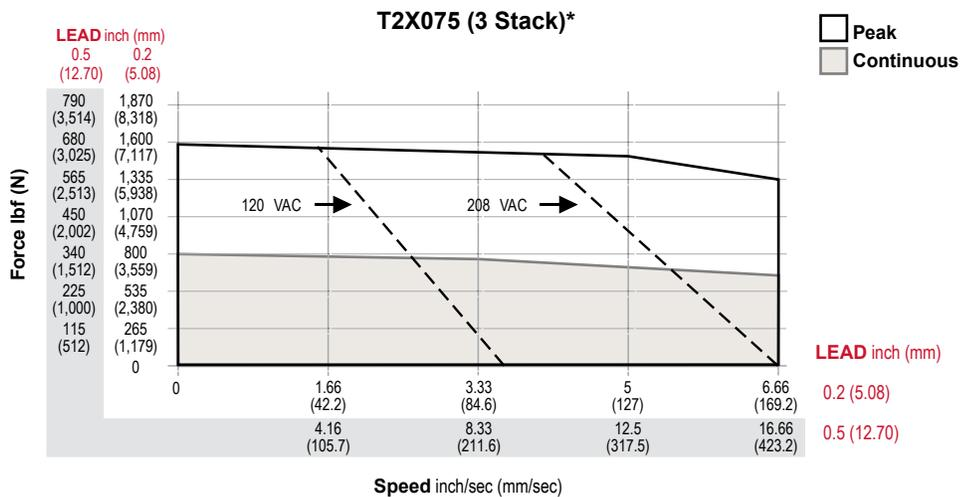
\*Test data derived using NEMA recommended aluminum heatsink 10" x 10" x 3/8" at 40°C ambient.
