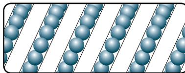
**Speeds:** Typical ball screw speeds are limited to 2000 rpm and less, due to the interaction of the balls colliding with each other as the race rotates. In contrast, the rollers in a roller screw are
