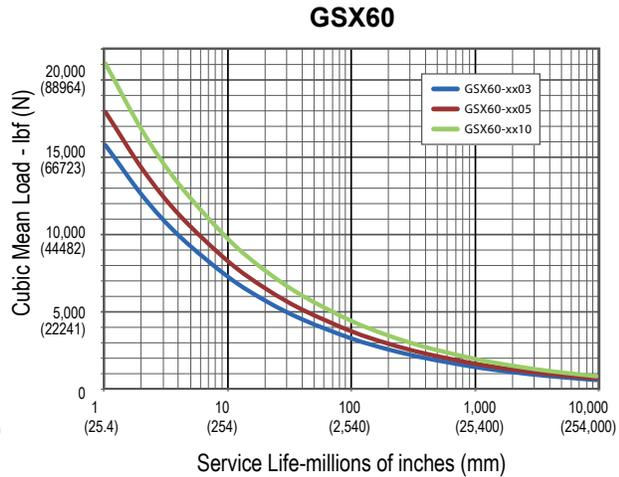
The  $L_{10}$  expected life of a roller screw linear actuator is expressed as the linear travel distance that 90% of properly maintained roller screws manufactured are expected to meet or exceed. This is not a guarantee and these charts should be used for estimation purposes only.
