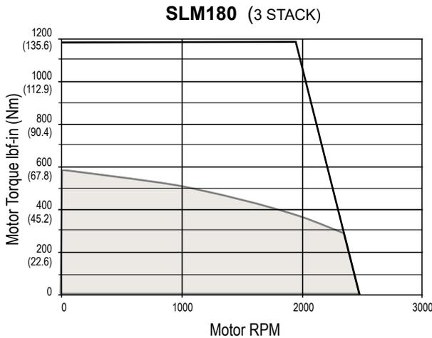
Test data derived using NEMA recommended aluminum heatsink 16" x 16" x 1" on SLM180 at 25°C ambient
