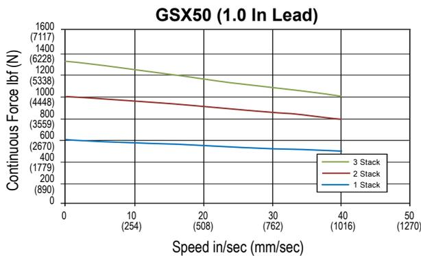
Test data derived using NEMA recommended aluminum heatsink 12" x 12" x 1/2" for GSX40, 12" x 12" x 1/2" for GSX50, and 16" x 16" x 1" for GSX60. Testing ambient temperature 25°C.
