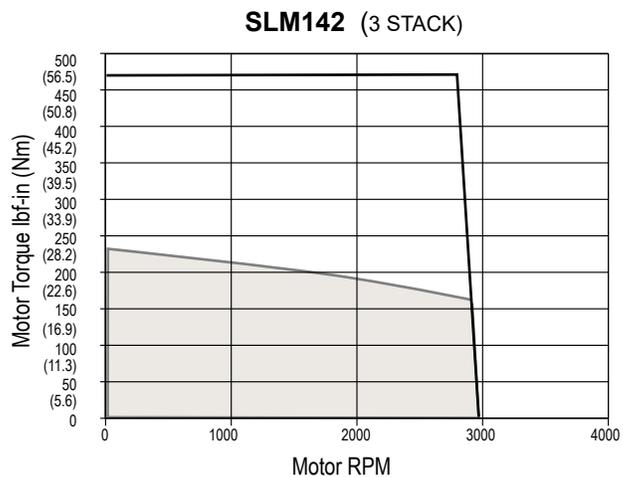
Test data derived using NEMA recommended aluminum heatsink 12" x 12" x 1/2" on SLM/SLG115 and 12" x 12" x 1/2" on SLM142 at 25°C ambient. For gearmotors, divide speed by gear ratio; multiply torque by gear ratio and efficiency. Efficiencies: 1 Stage = 0.91, 2 Stage = 0.86
