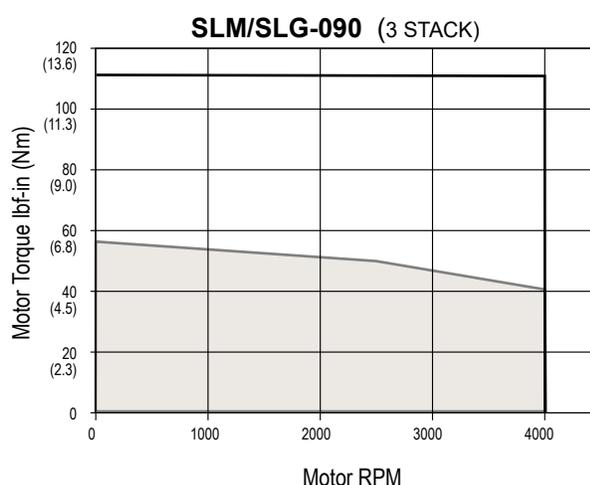
Test data derived using NEMA recommended aluminum heatsink 10" x 10" x 3/8" on SLM/SLG075 and 10" x 10" x 3/8" on SLM/SLG090 at 25° C ambient. For gearmotors, divide speed by gear ratio; multiply torque by gear ratio and efficiency. Efficiencies: 1 Stage = 0.91, 2 Stage = 0.86
