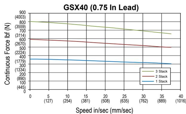
Test data derived using NEMA recommended aluminum heatsink 10" x 10" x 1/4" for GSX20 and 10" x 10" x 3/8" for GSX30. Testing ambient temperature 25°C.
