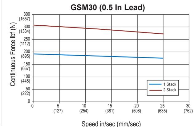
Test data derived using NEMA recommended aluminum heatsink 10" x 10" x 1/4" on GSM20 and 10" x 10" x 3/8" on GSM30
