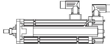
The external limit switch option (requires anti-rotate option) provides the user with 1, 2, or 3 externally mounted adjustable switches for use as the end-of-travel limit switches or home position sensors.
