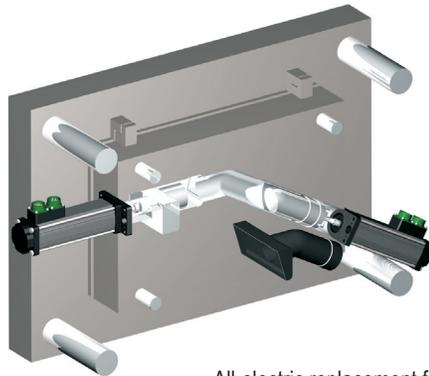
All-electric replacement for hydraulic cylinders improves throughput with servo control and lower maintenance for core-pull cylinders.
