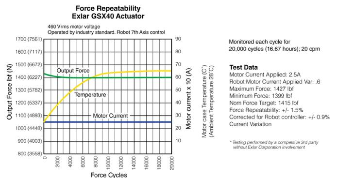
This data demonstrates the excellent force repeatability available to you in an open loop system. If your application requires even more accurate force control Exlar offers integrated force sensing devices for monitoring force in your application.
