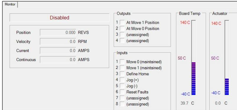
This screen shows actuator status along with position / velocity / current information. The digital input/output line statuses may also be viewed along with the board and actuator temperatures.
