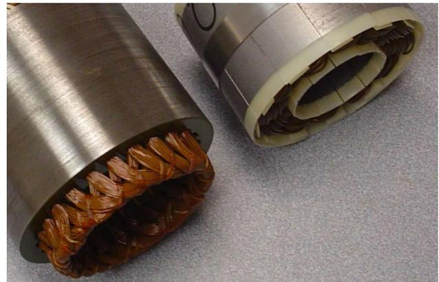
Figure 4: End turn length comparison
