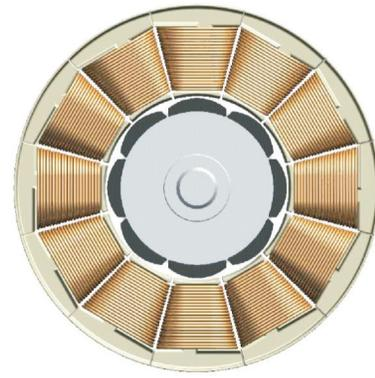
Figure 3: Minimized, non-overlapping end turns
