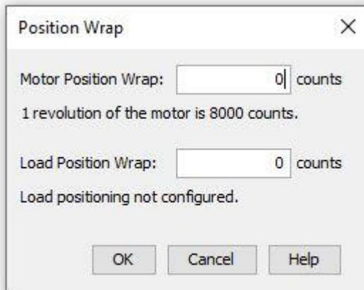
Change/verify the position wrap parameters as needed. Set both values to zero to disable position wrapping. Note that the changes do not take effect until **OK** is pressed. For more information about this feature, see Position Wrap.
