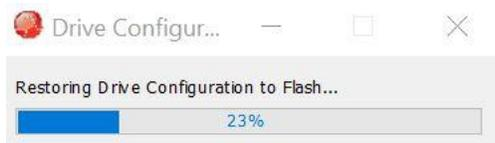
All the data read from the file is saved to the drive's Flash. After all the data is written, the drive will be reset, so that the Flash data is copied to RAM.
