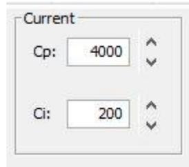
7. Adjust current loop integral gain ( $C_i$ ) until desired settling time is obtained.
