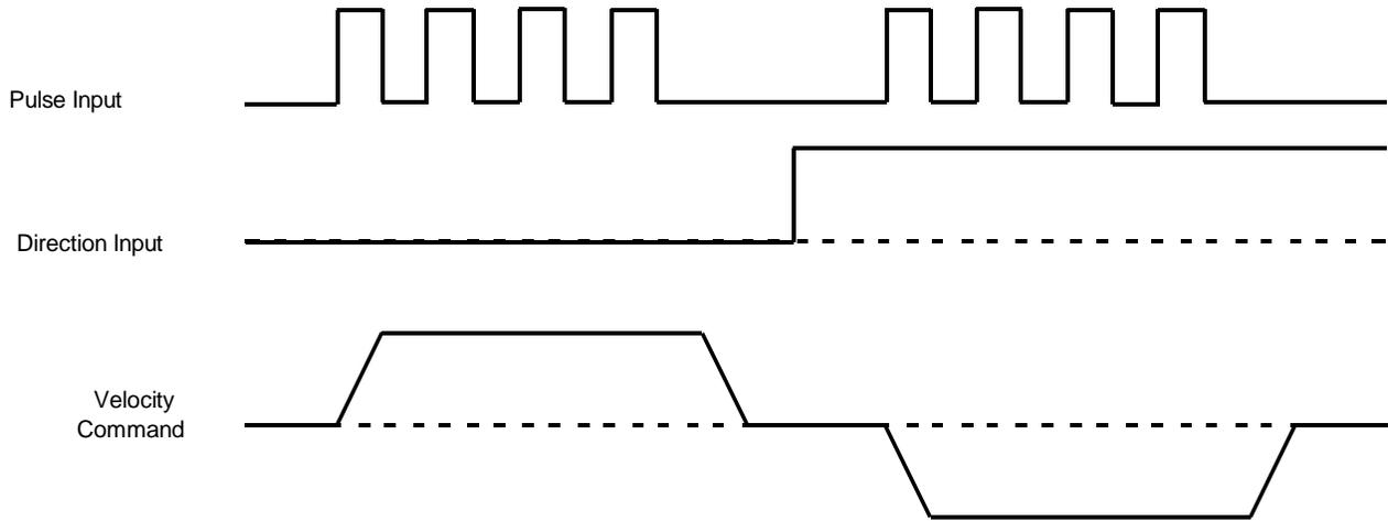
The amplifier can be set to increment position on the rising or falling edge of the signal. Stepping resolution can be programmed for electronic gearing.
