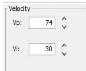
7. Adjust velocity loop integral gain ( $V_i$ ) until desired settling time is obtained.
