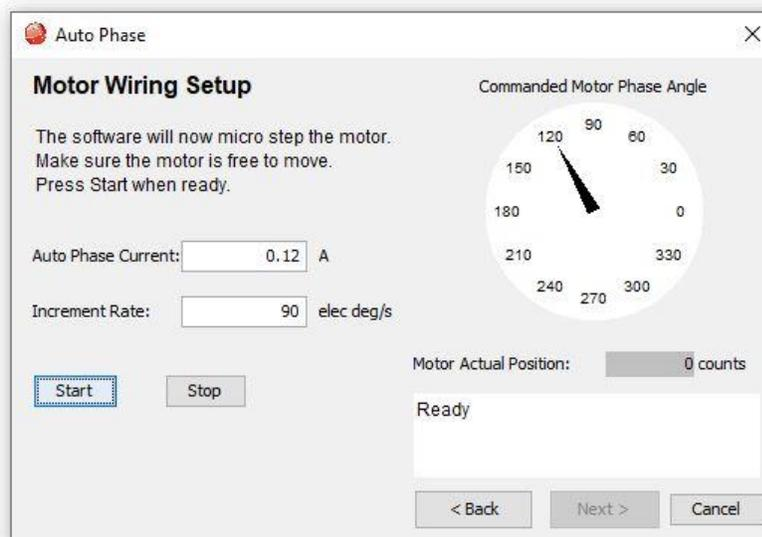
6. Click **Start** to begin motor wiring setup with default values. After successful motor wiring setup, the message "Test Complete" appears.
