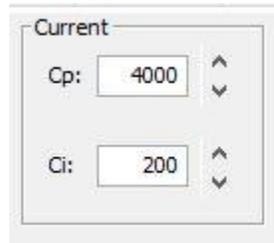
17. Adjust current loop integral gain (Ci) until desired settling time is obtained.
