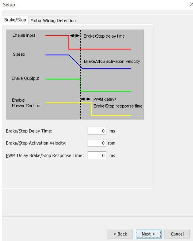
Many control systems employ a brake to hold the axis when the amplifier is disabled. On brake-equipped systems, disabling the amplifier by a hardware or software command starts the following sequence of events.
