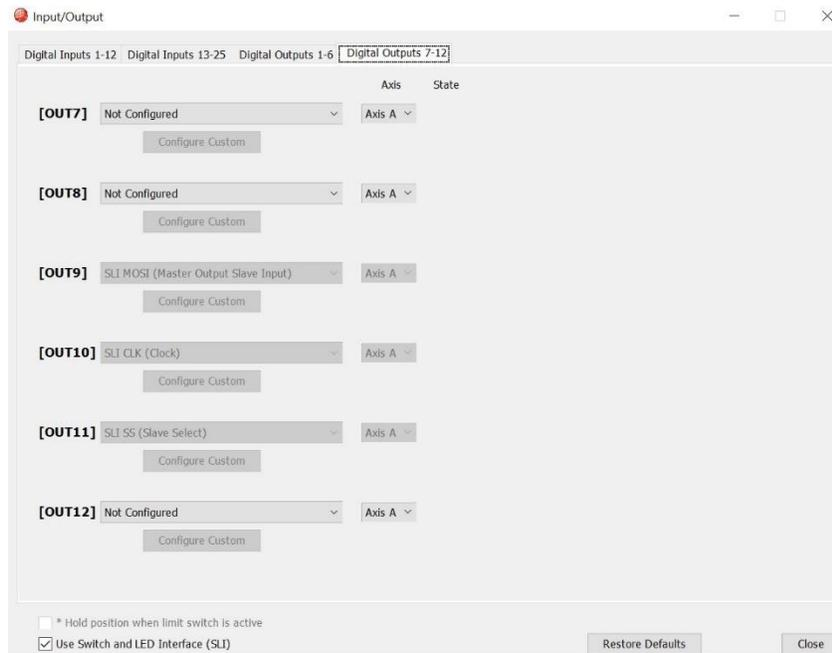
Uncheck the box to disable Network ID switch and LED to get additional I/O (3 outputs, 1 input).
