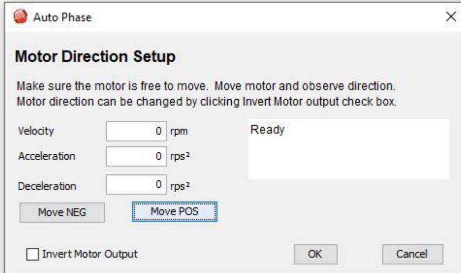
3. Hold down **Move POS** to move the motor in the direction considered positive and observe the direction of movement.
