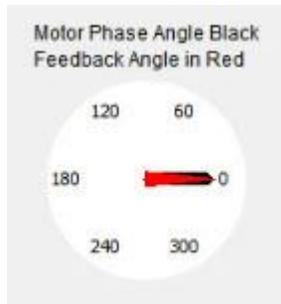
Note: Motor manufacturers typically align the resolver in 30 degree increments, typically by applying current through a pair of motor power wires.
