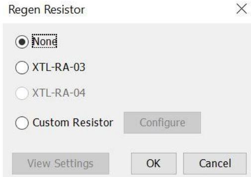
2. Select Custom Resistor and click **Configure** to enter the custom resistor data. Read the information displayed and click **OK**.
