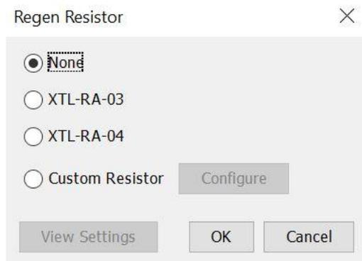
2. Select the model number XTL-RA-03 or XTL-RA-04 based on your drive and click **OK** to save the configuration and close the screen.
