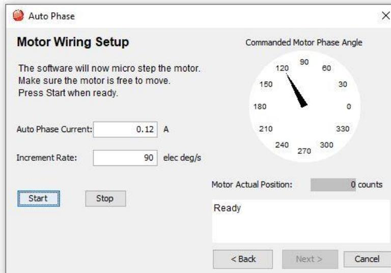
6. Click **Start** to begin the motor wiring setup. The message area displays messages: Configuring Initial Settings, Microstepping, Test Complete, Motor Wiring has been configured.
