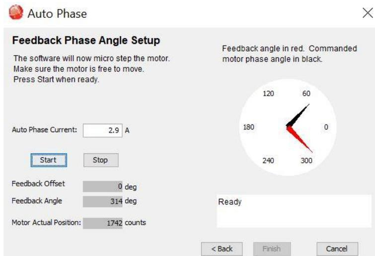
13. Click **Start** to start the resolver phase angle setup. The message area displays status messages.
