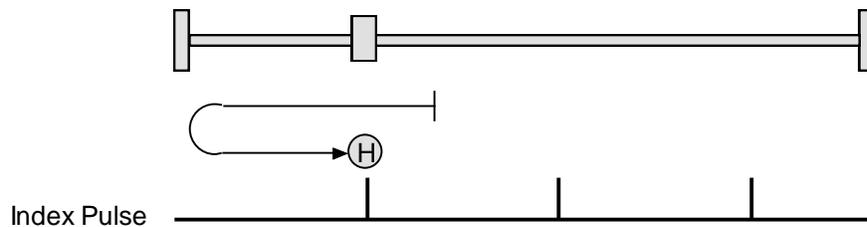
**Hardstop Out to Index Methods in Stepper Mode**
