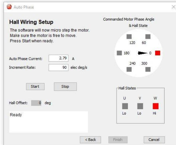
11. Click **Start** to begin the Halls wiring setup. The message area displays the messages: Microstepping. Test Complete. Motor has been properly phased.
