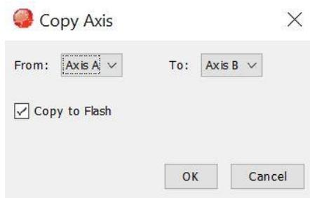
Select the source and destination axes, then click **OK**. Note that Copy to Flash is selected by default. If this option is not selected, then the RAM/Flash parameters will only be copied to the destination axis' RAM, while still copying the Flash Only data to the destination axis' Flash.
