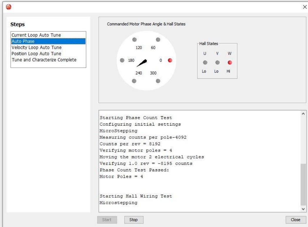
5. When the auto phase is complete, it goes to **Velocity Loop Auto Tune**.
