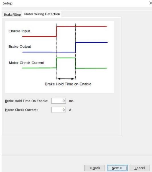
On some drives, the amplifier can check for a disconnected motor. Upon enable, the amplifier will apply current to the motor windings, while keeping the brake engaged for the brake hold time. If the current vector cannot be applied, then a motor disconnected fault will occur, and the brake will not be released. If the motor is connected, the brake will be released after the brake hold time expires.
