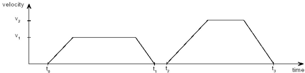
The *CANopen Profile for Drives and Motion Control (DSP 402)* refers to this method as the “single set point” method.
