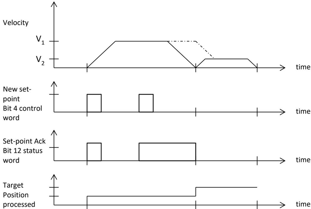
The dashed line in the first graph represents the velocity if the *change of set point bit* (bit 9 of the control word) is set.
