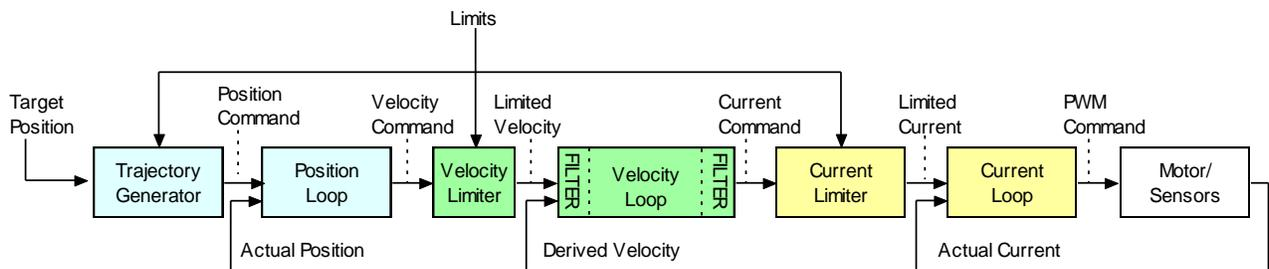
In velocity mode, the velocity loop drives the current loop. In current mode, the current loop is driven directly by external or internal current commands.
