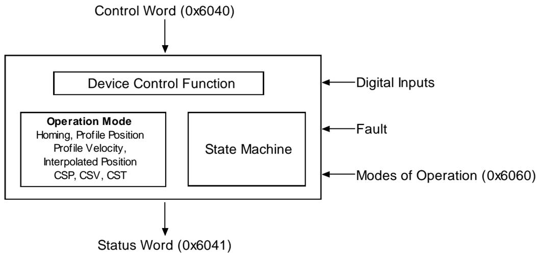
Other factors affecting control functions include: digital input signals, fault conditions, and settings in various dictionary objects.
