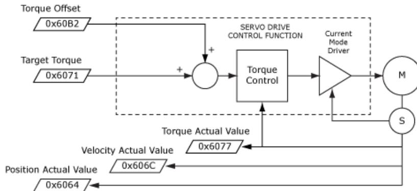
This diagram shows the CST control function with real-time and other configuration parameters.
