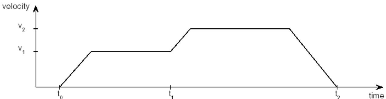
The *CANopen Profile for Drives and Motion Control (DSP 402)* refers to this method as the “set of set points” method.
