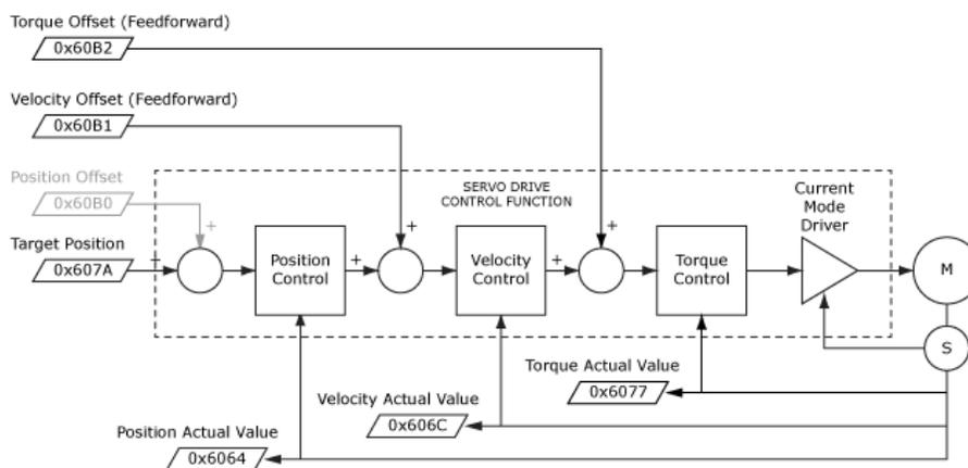
This diagram shows the CSP control function with real-time and other configuration parameters.
