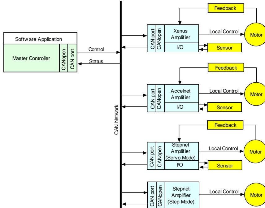
A CANopen network can support up to 127 nodes. Each node has a seven-bit node ID in the range of 1-127. Node ID 0 is reserved for the master and slave addresses can be 1~127.
