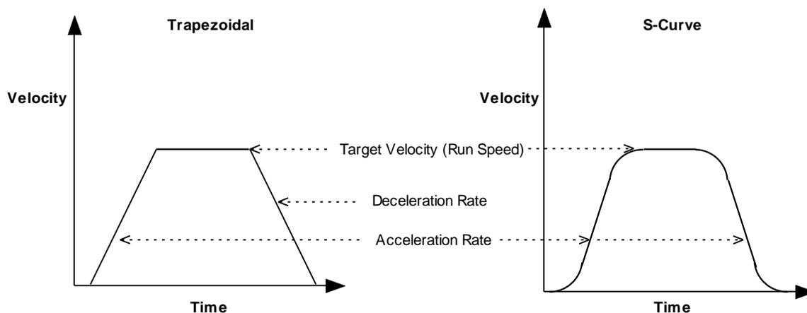
In a trapezoidal profile, jerk is unlimited at the corners of the profile (start of the move, when the target velocity is reached, when deceleration begins, and at the end of the move). S-curve profiling limits jerk or “smooths” the motion.
