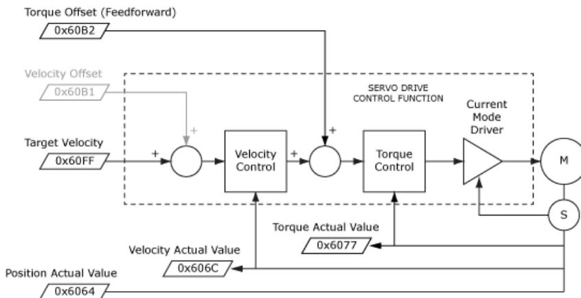
This diagram shows the CSV control function with real-time and other configuration parameters.
