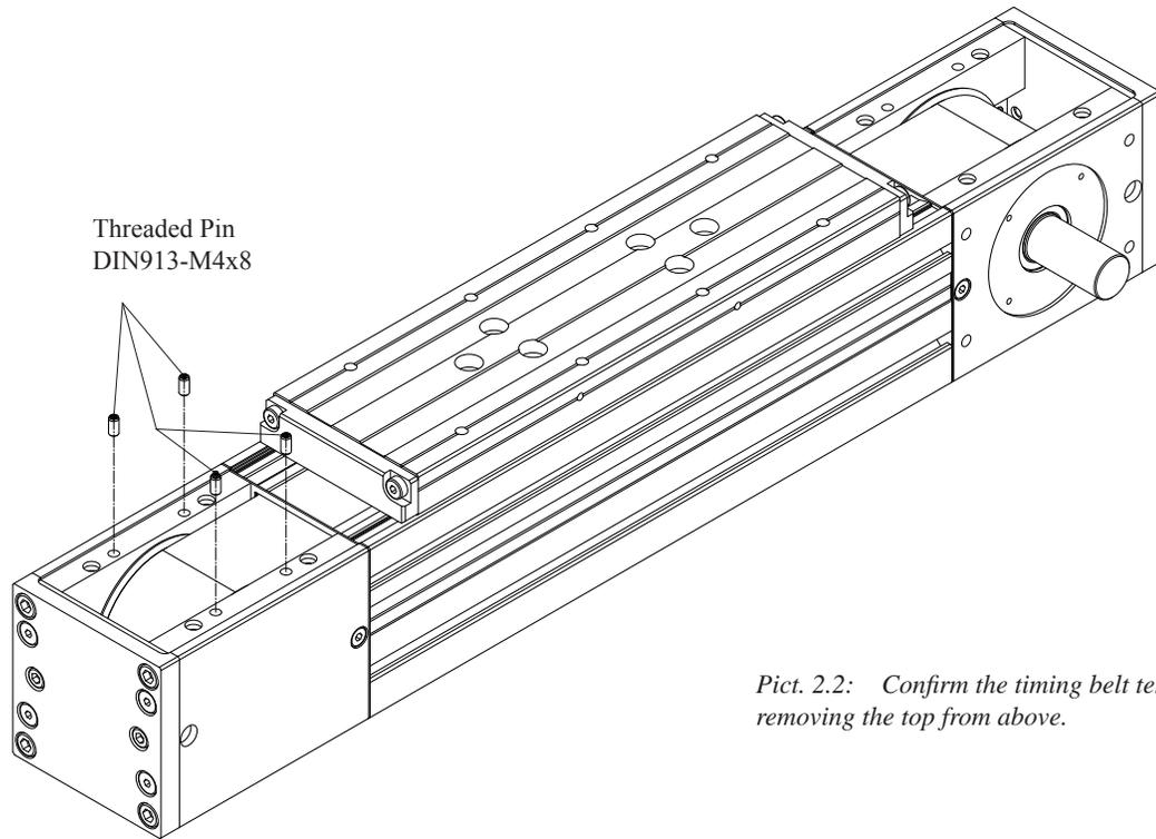
*Pict. 2.2: Confirm the timing belt tension by removing the top from above.*
