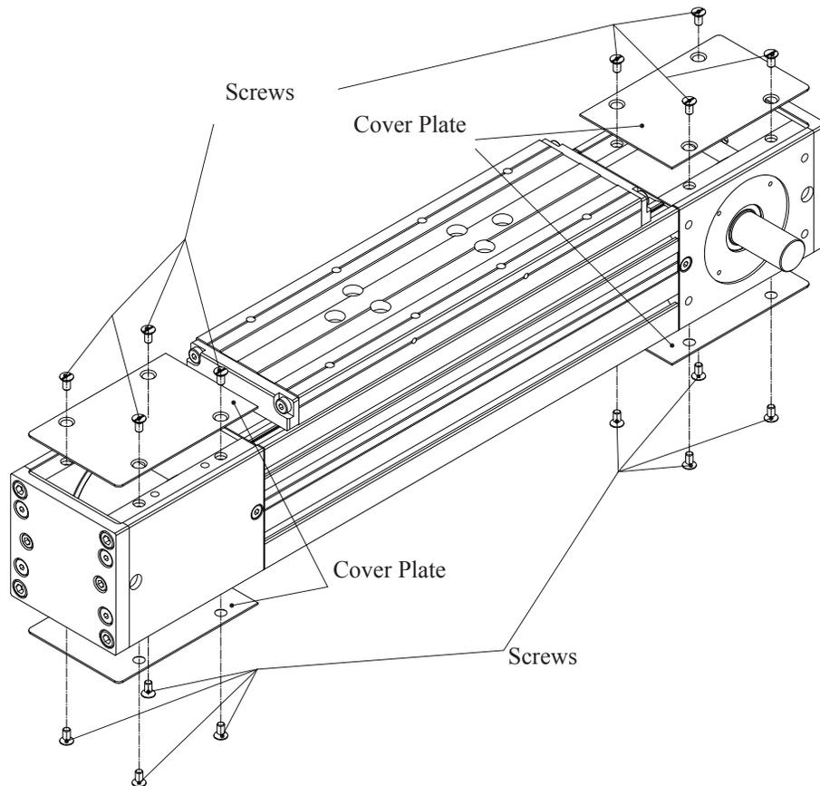
Turn out the screws and remove cover.
