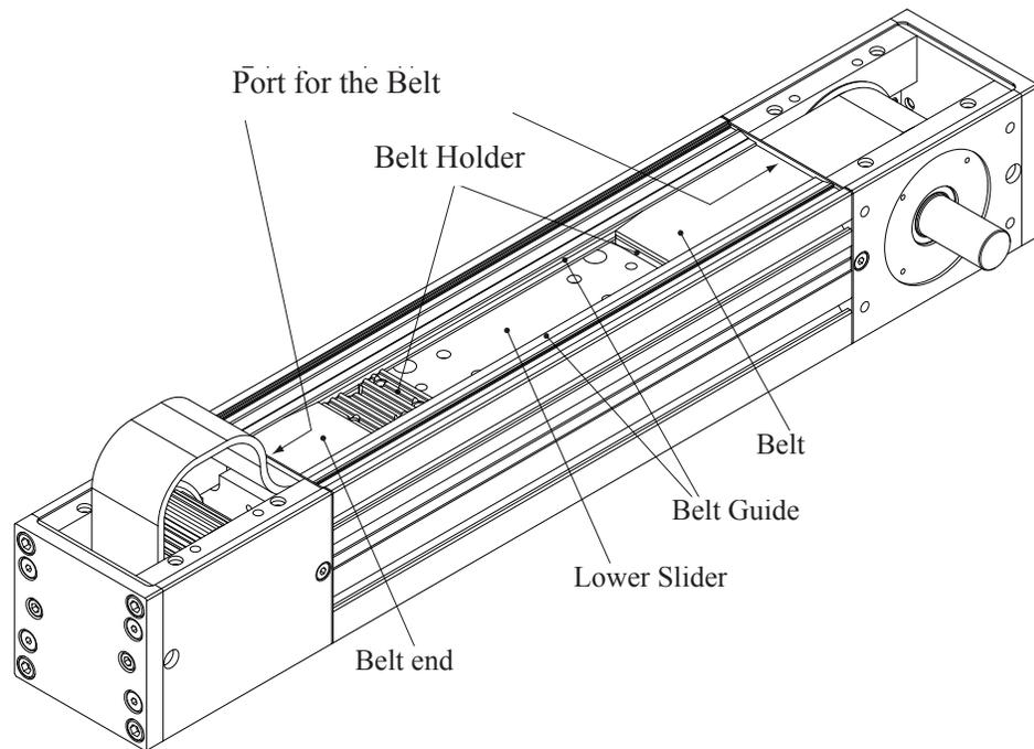
Lift belt ends and remove through the ports.
