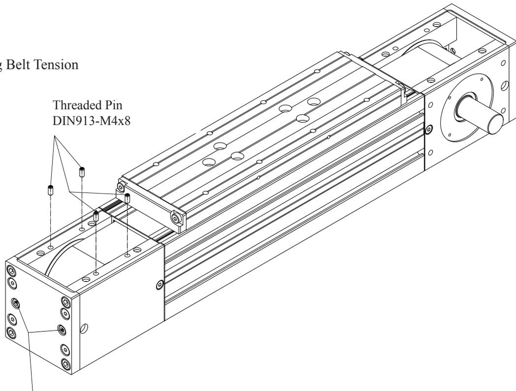
Use these screws to adjust belt tension, take care that both are turned equal.
