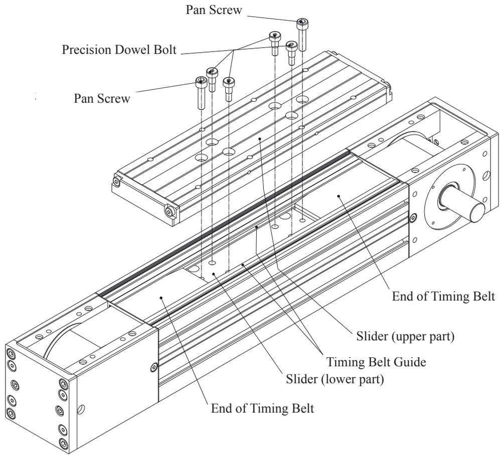
Remove all screws and remove the upper part of the slider.
