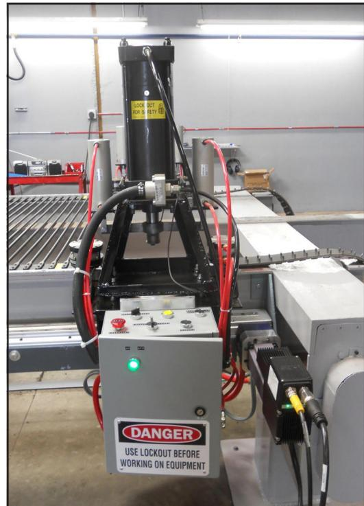
*Exlar's Tritex II rotary actuator installed on automated riveting machine*
