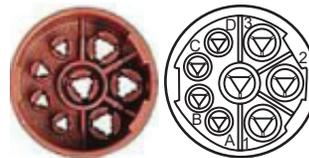
Power Connections on Terminal board 80 mm
