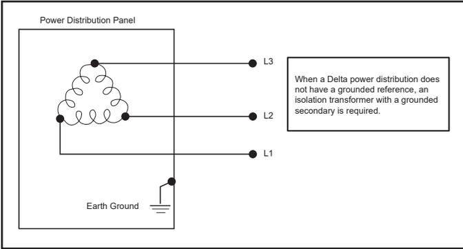
**Figure 18 – Ungrounded Delta Power Distribution**
