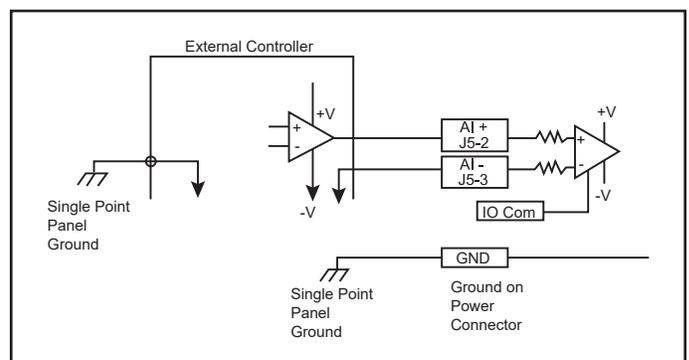
**Figure 32 – Analog Input Wiring from External Controller**
