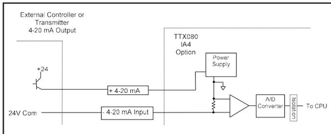
Figure 36 – Connection to High Side Controller
