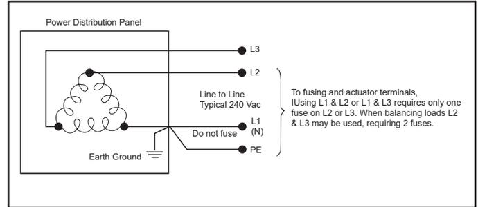
Figure 15 – Three Phase Grounded Delta Power Connection, 240 VAC
