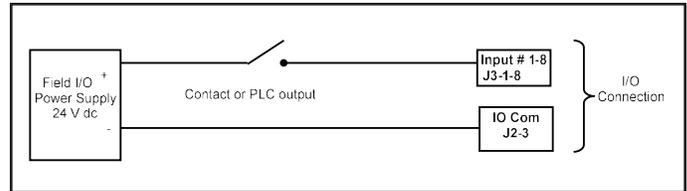
Figure 26 – Input Wiring with External 24Vdc Power Supply
