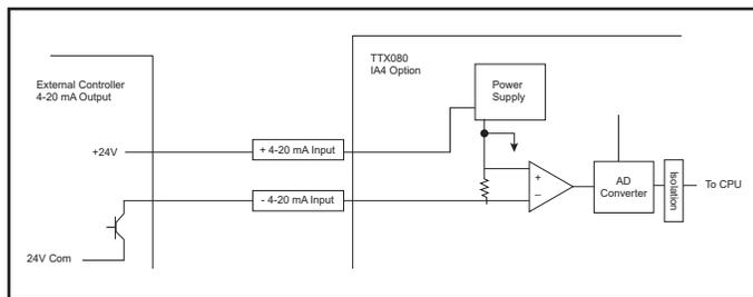
Figure 37 – Connection to Low Side Controller
