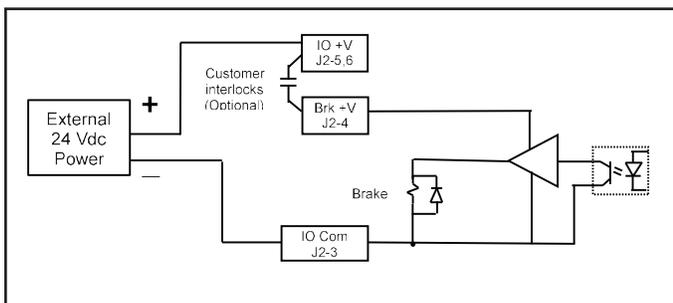
**Figure 30 – Brake Connections with External 24V Power Supply**
