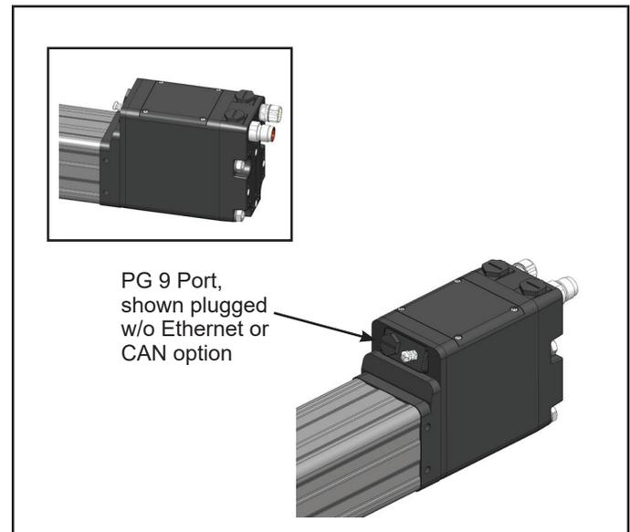
Figure 11 – PG9 Cable Entry Port / Communication Connector
