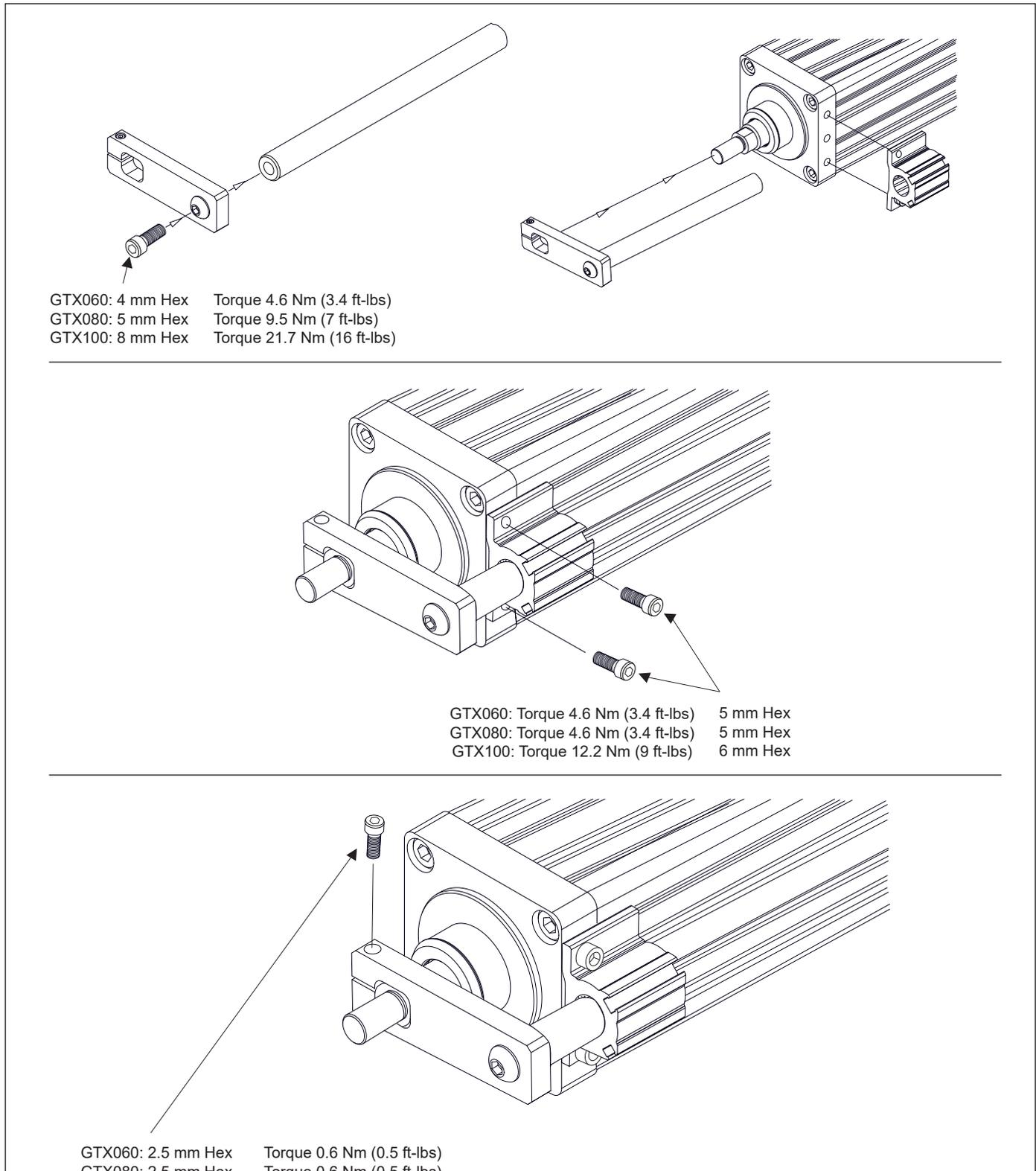
Figure 6 – Anti-rotation Assembly (shown in standard location)
