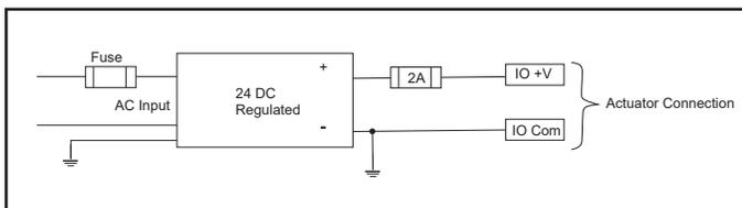
**Figure 22 – Wiring for External 24 Volt Supply**
