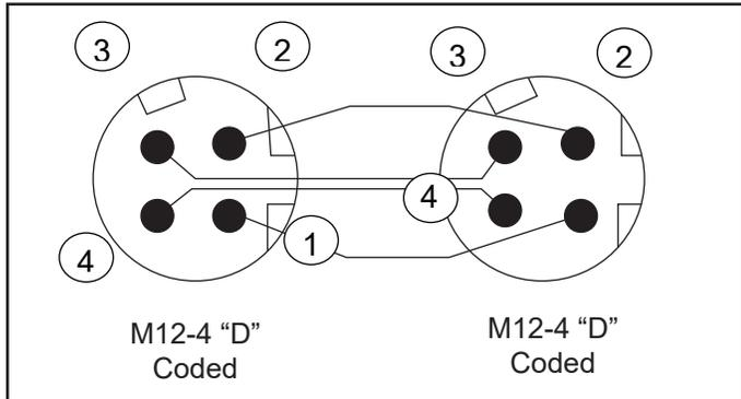
**Figure 39 – M12 D Coded Straight Through Cord Set**
