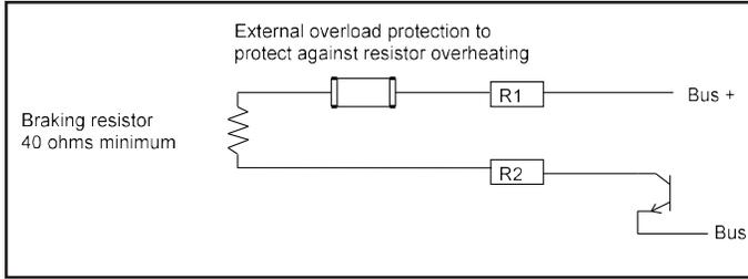
**Figure 21 – Braking Resistor Connections**
