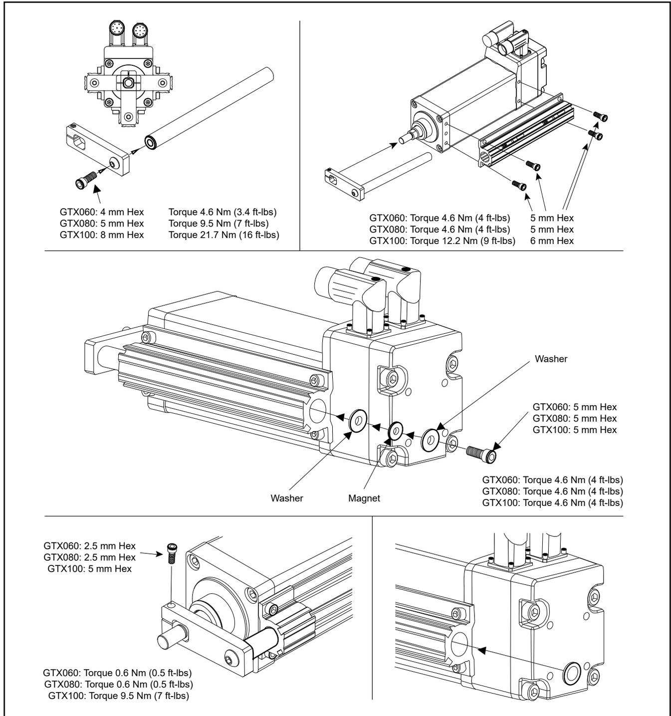
Figure 7 – Limit switch mounting
