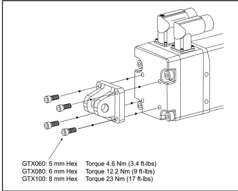
**Figure 3 – Rear clevis mount** (NOTE: Dimension drawings can be found in the GTX Series Actuator catalog or on the Exlar website.)
