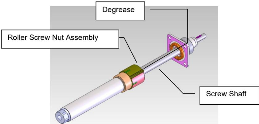
**Lubrication**—The planetary roller screw shaft or acme screw shaft and nut assembly, anti-rotates, linear bearing, and rotary seal are factory lubricated. The anti-rotate and linear bearing does not need re-lubrication. If the roller screw shaft or acme screw shaft need re-lubrication, follow the disassembly process for the actuator in Section 3.8 Disassembly & Reassembly Procedure.
