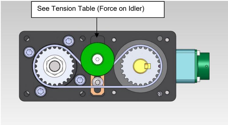
The idler pulley plate slot allows moving the idler pulley so the belt can be placed, followed by placing a force directly over the idler pulley to obtain the proper tension to tighten the belt (See table next page).
