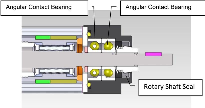
**Figure: Roller Screw Support Using Angular Contact Bearings**
