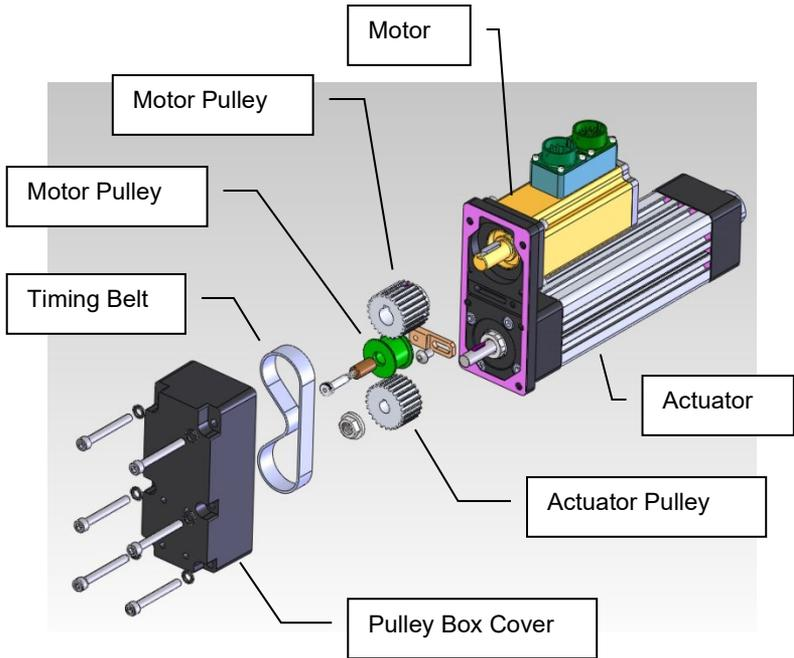
**Figure: Parallel Motor Mount Drive Train Assembly**
