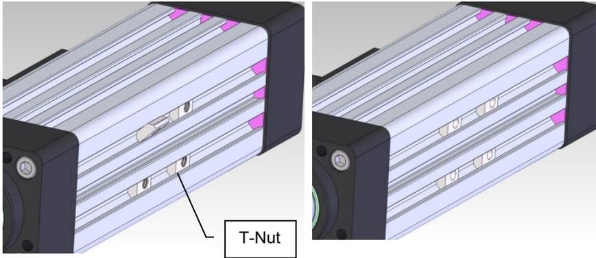
**Step 1:** Insert T-nuts at an angle into the t-nut rail slot.
