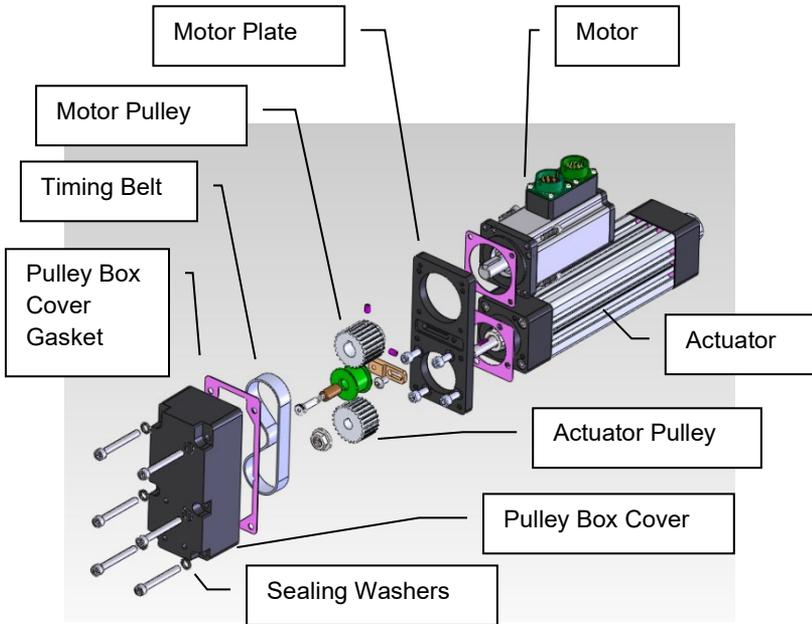
*Figure: Parallel Motor Mount Drive Train Assembly*
