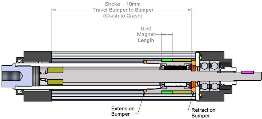
*Figure: Actuator Shown in fully retracted “crash” position, with contact on the Retraction Bumper*
