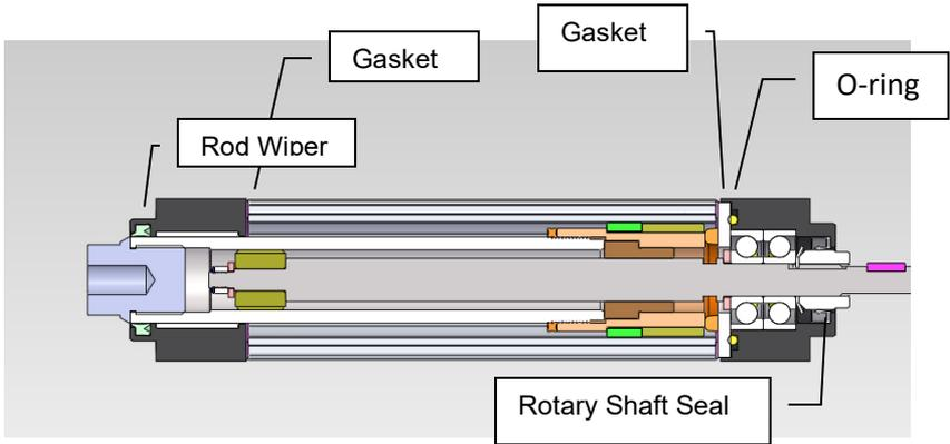
**Figure: Base Unit Sealing Details**
