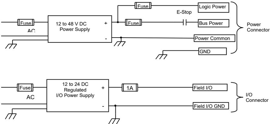
*Two Power Supply Configuration, Maintaining I/O Isolation*
