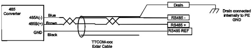
*Typical RS485 connection to external converter*
