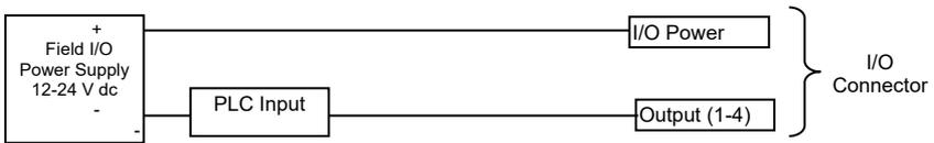
*External Wiring of Outputs for Connection to PLC or Any Load*
