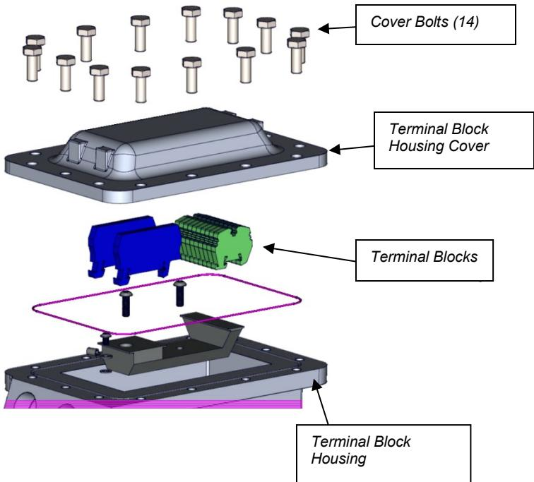
All connections to the terminal box inside the housing are made as indicated in the diagram below. When the terminal box cover is removed, the installer can have access to the wiring connections. As indicated on the actuator label "KEEP COVER TIGHT WHILE CIRCUITS ARE LIVE"
