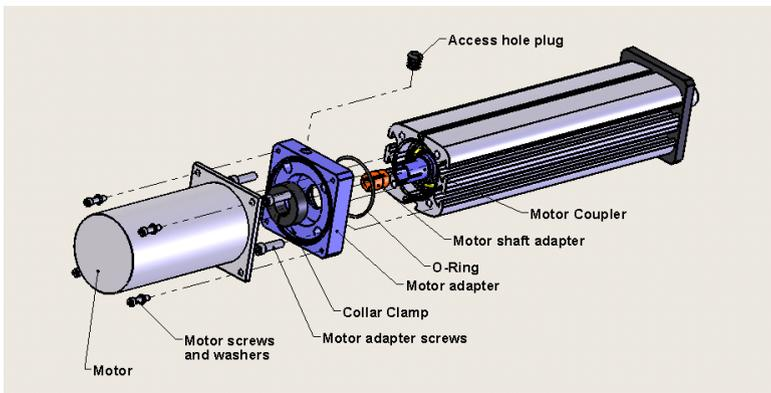
Figure 12: Inline Motor Mount Disassembly
