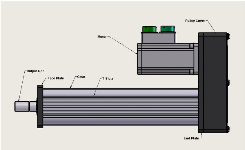
*Figure 3: I Series with Parallel Motor Mount*
