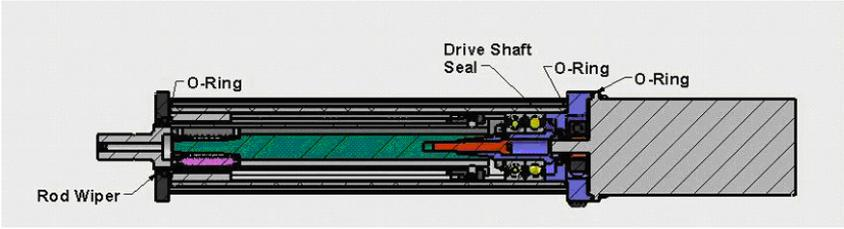
Figure 7-2: IP65 Integrated Motor Mount Unit Sealing Details
