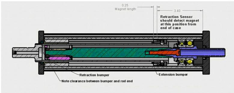
Figure 10-2: Actuator Shown in maximum recommended retract position, with 0.2” (5.08 mm) of clearance on forward impact bumper.
