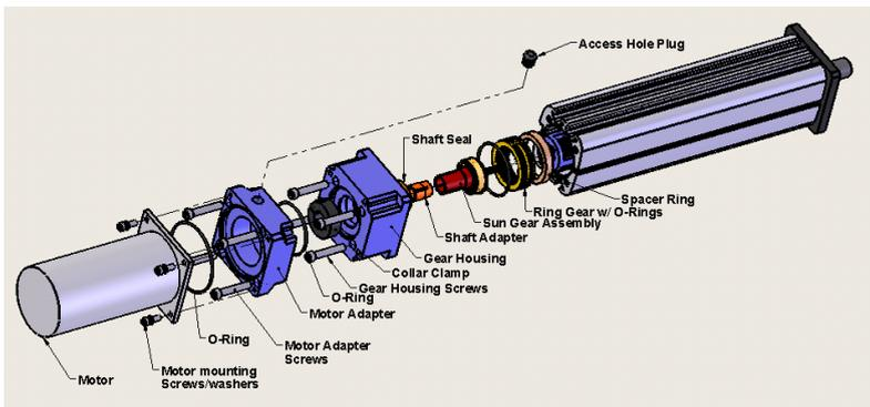
Figure 13: Inline gear set/Motor Mount Disassembly
