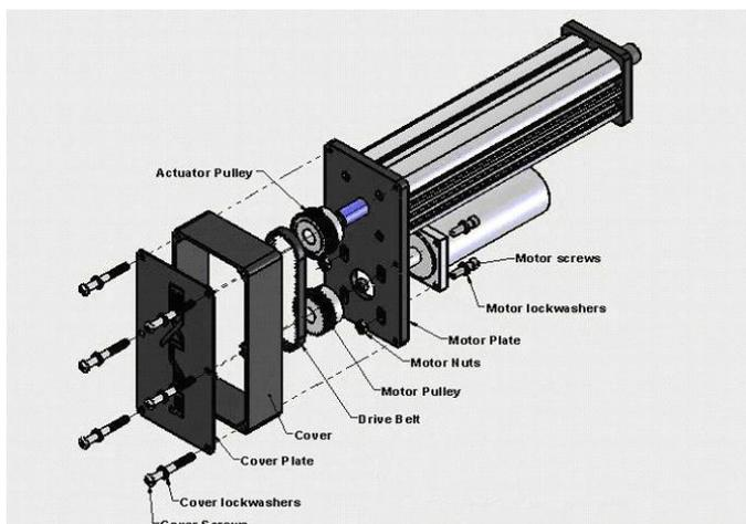
*Figure 9: Parallel Motor Mount Drive Train Assembly*
