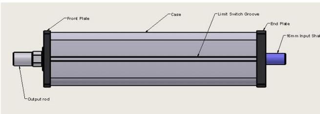
*Figure 2: I Series Base Model Actuator*
