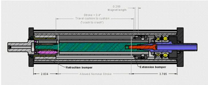
Figure 10-1: Actuator Shown in fully retracted “crash” position, with contact on forward impact bumper
