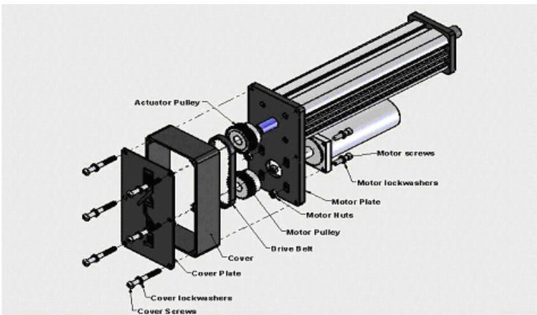
*Figure 11: Parallel Motor Mount Drive Train Assembly*
