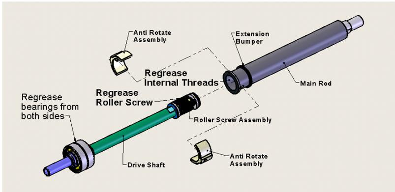
Figure 14: Actuator Disassembly
