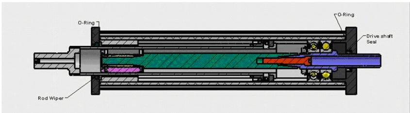
Figure 7-1: IP65 Base Unit Sealing Details
