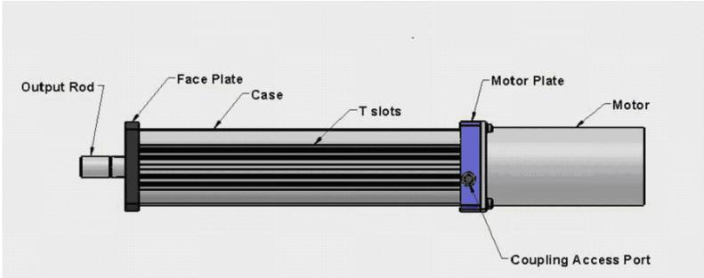
*Figure 4: I Series with Inline Motor Mount*
