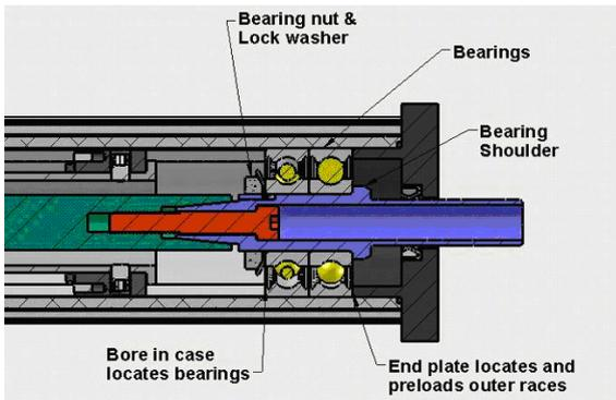
Figure 8: Roller Screw Support Bearing Detail
