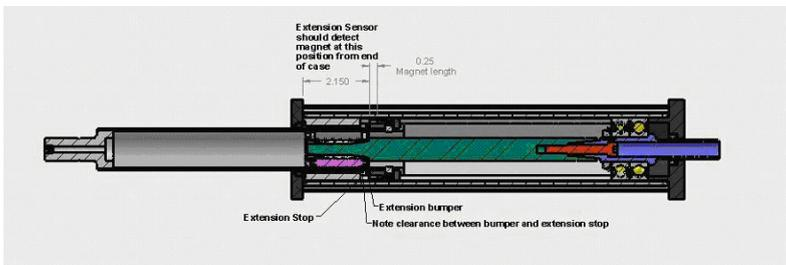
Figure 10-3: Actuator Shown in maximum recommended extension position, with 0.2” (5.08 mm) of clearance on aft impact bumper.
