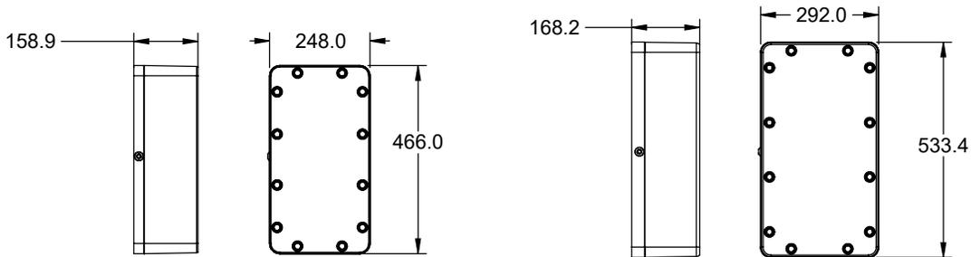
NOTE: 248mm Wide Housing used for Motors with 215mm Mounting B.C. and Smaller P10 1:1 Mounts,
