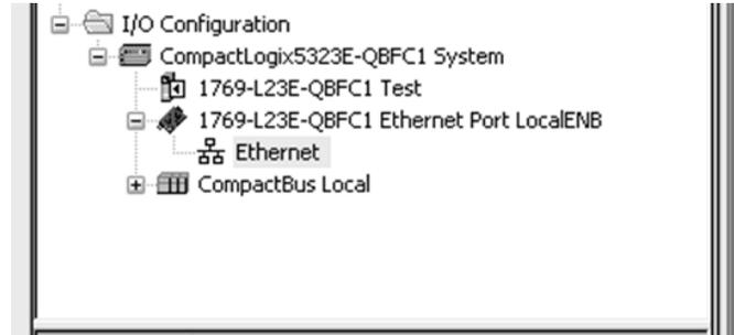
Figure 17 – Adding a New module using PLCs Software
