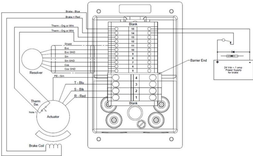
Note 1: Thermal switch normally closed; opens when stator temp exceeds 130 deg. C.
