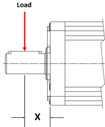
Figure 3-3 Radial Loading
