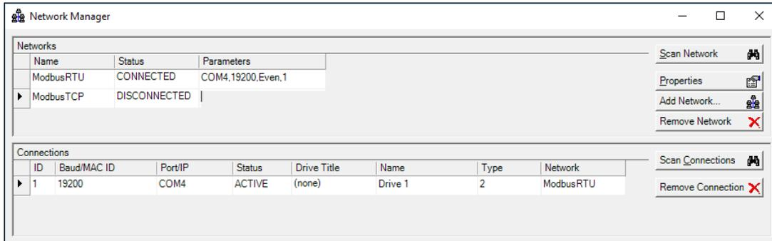
Above image is after 'Scan Network' and Ethernet Network interface not detected. This is not a likely result, but needs to be fixed in the PC first. More likely there will be one or more IP addresses. However if nothing shows up in the Connections area as shown above, there is a problem with the Ethernet link between PC and actuator. Make sure network status LED's are green and the PC Network Interface Status is OK. Make corrections as needed and scan again.
