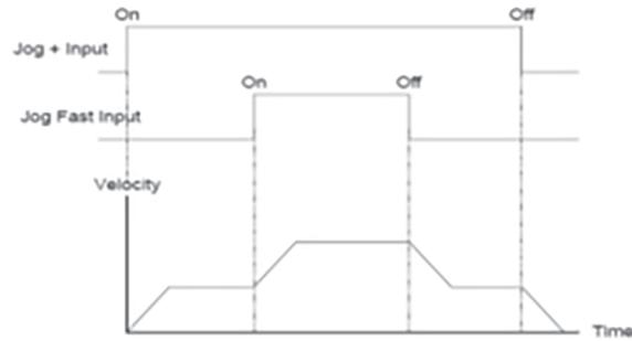
The *Jog* function can be initiated from the *Jog +/-* input functions, which can be activated from the assigned digital inputs, *Input Function Control* page, *Jog* buttons on the *Jog* page or the *Control* page, or from a Modbus command. *Jog* can be selected to override other motion types as well. (See the *System Setup* page description and *Motion Description* section).
