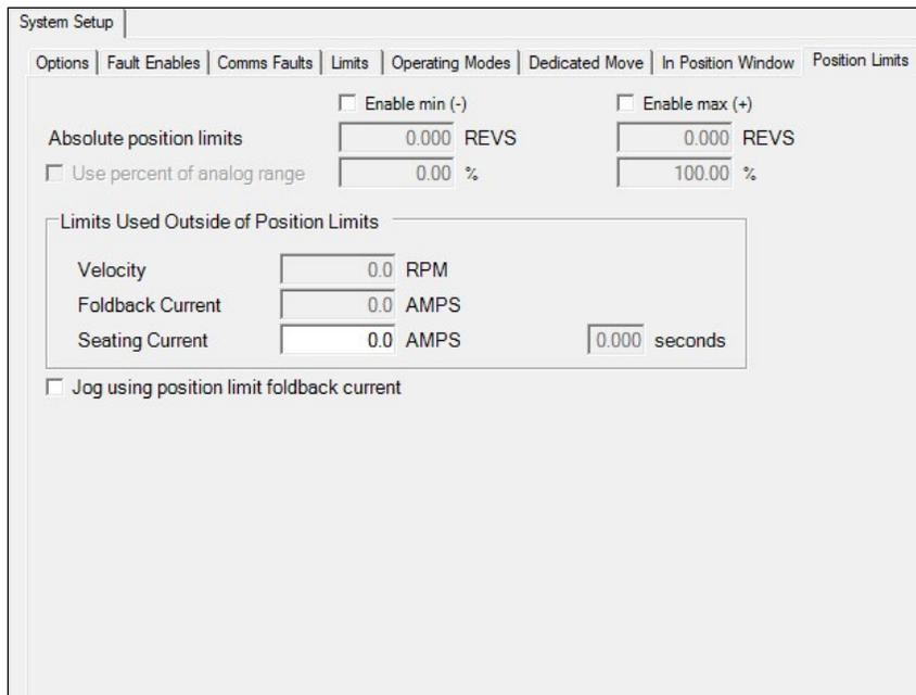
*Position Limits* are software monitored travel limits, with special features for control outside of these travel limits.
