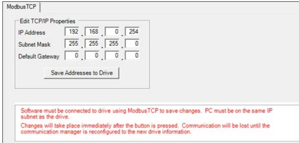
After saving to drive, the connection will be lost immediately. Many times there is no further reason to connect to the drive via the ModbusTCP network from Expert Software. The connection can be accessed over the ModbusRTU network. Reconnection is possible over ModbusTCP, but the Network Interface may have to be changed to the new subnet, and the network will need to be scanned again.
