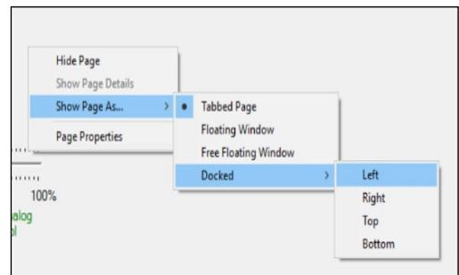
Also pertinent to page appearance is the bottom of the *Page Properties* window that appears when clicking on that entry. *AutoScroll* allows a page larger than the main body area to scroll as needed to see the entire page. *Detail Page* simply means it does not appear until requested. *Show in page drop-down lists* means it appears in the *System Panel*.
