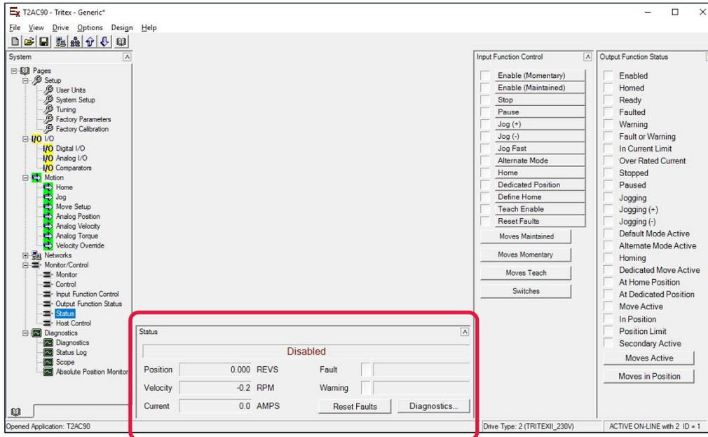
Referring to the image above, *Disabled* is the current operating state of the actuator.
