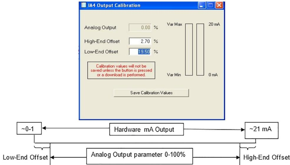
The actual hardware output is designed to allow an output span that is greater than 4mA to 20 mA, this assures that 4-20 mA can always be delivered to the Host considering all component tolerances and other losses before the signal gets to the host controller.
