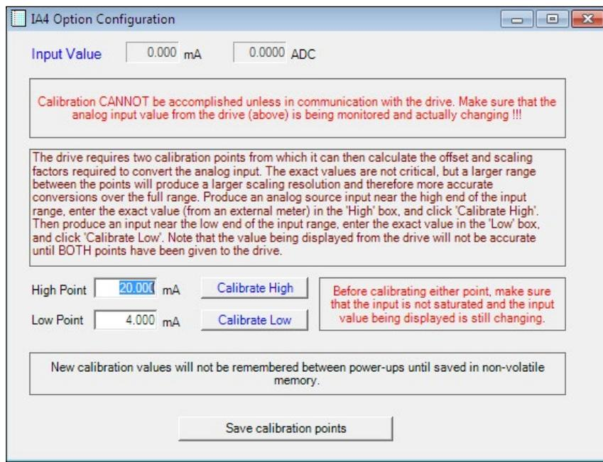
A Loop Calibrator instrument that provides loop power and an accurate current is very useful for calibrating a 4-20 mA input. The input is best calibrated at 4 mA and 20 mA.
