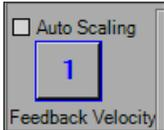
This button, whose number changes as it is toggled, selects which channel will be affected when the *Scale* or *Offset* slide bars are used. This is also the channel that the values displayed on the vertical grid line will represent.
