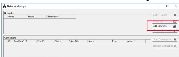
Click on the *Add Network* button. The window shown on the right pops up. Select *ModbusRTU* from the drop-down and OK.
