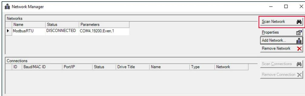
When Expert finds a device or devices connected to the configured COM port, the connections will appear in the Connections section with Status = ONLINE. This does not mean it is Connected and actively communicating to the actuator; only that the connection is available.
