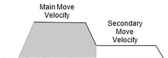
Main move with secondary motion enabled.
