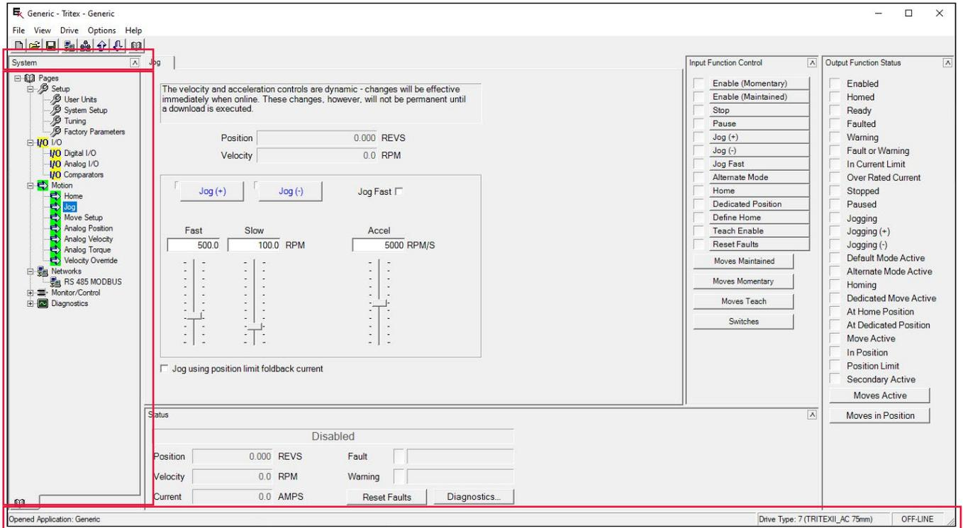
Use the *View* drop-down menu to show or hide the special bars and panels by clicking on the name. Pages may also be shown from the available pages sub-menu shown expanded here, though these are generally selected from the *System Panel*.
