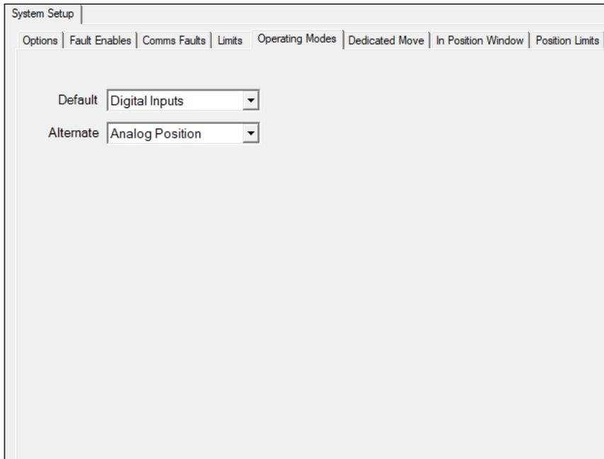
This tab allows selection of the source/motion type for *Default* and *Alternate* modes. The description of these modes of operation are available by right clicking on the drop box and selecting the View Helpfile. The possible selections for each mode include:
