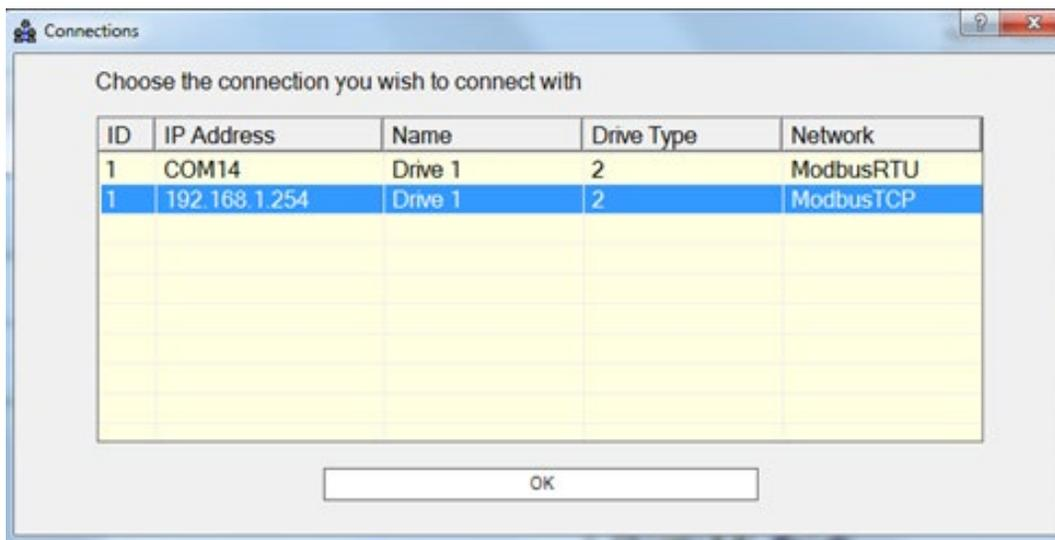
If the IP address is to be changed to connect into the end use network, open the ModbusTCP page from the Networks group. Type in the new IP address and other parameters as needed and click on the Save Addresses to Drive button.
