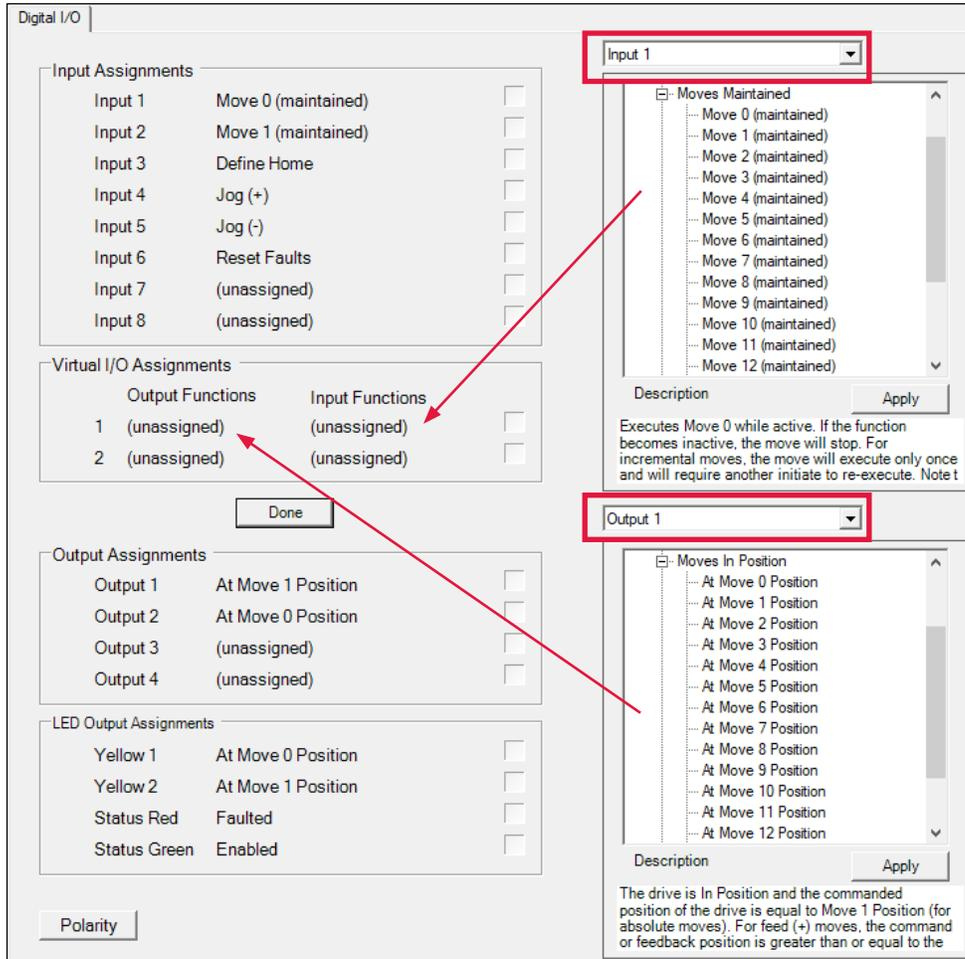
The *Virtual I/O Assignments* section allows an output event to set or clear and input event. By selecting either Virtual Output 1 or 2 from the Output Assignments tab, a given output event can be selected. Likewise, by selecting either Virtual Input 1 or 2, from the Input Assignments tab, a given input event can be selected. Feature added with Tritex II AC 90/115 mm v2.21 and Tritex II DC and AC 75 mm v2.37. Not available on EXP-24.
