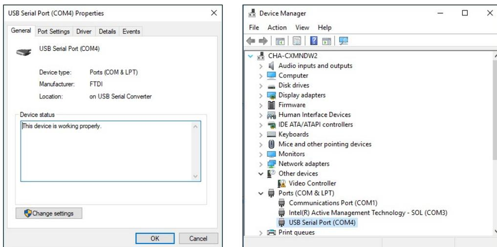
The name of the device driver installed must show under Ports. If it does not, the Expert software cannot connect to the PC COM port. COM4 is used in the example above. Use the correct COM port number in the Expert software when setting up PC communication. Double-click on the COM port to see the screen above on the right to verify the converter's device driver is working.
