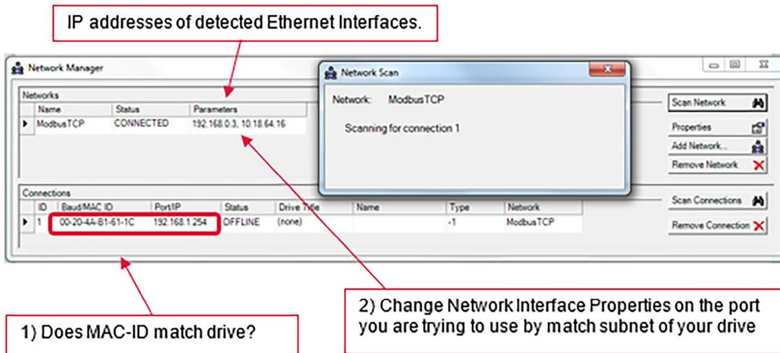
The above images show a device was found but it was on a different subnet, so could not connect. Check that the MAC ID is the actuator to be connected. Change PC Ethernet network properties to match found actuator subnet, meaning the first three numbers match. Then press *Scan Connection* button again.
