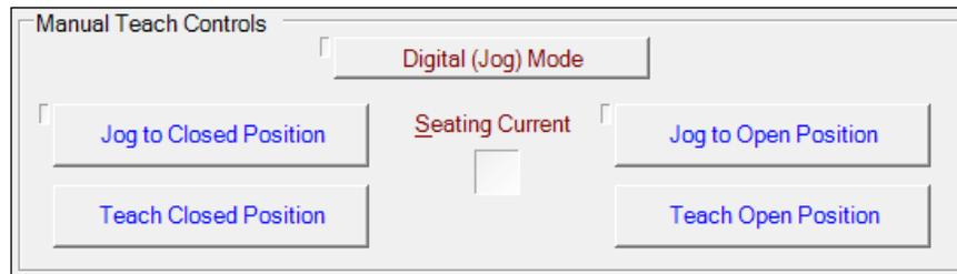
Selecting *Digital Jog Mode* allows the valve to be manually jogged to its closed and open positions. Click on the *Digital Jog Mode* button to enable this feature.
