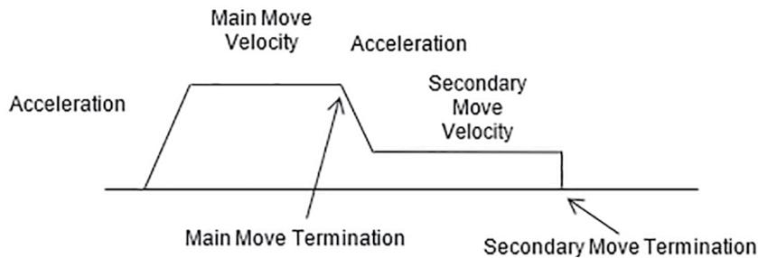
**Moves ended with a termination of switch or current limit**
