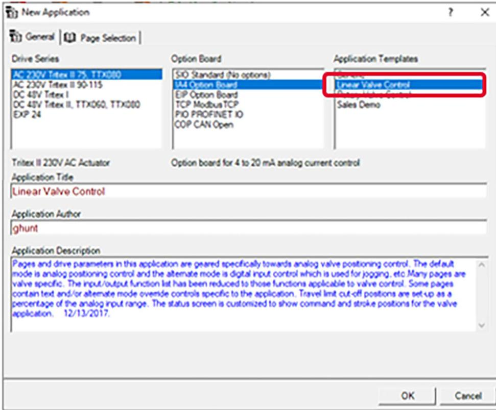
Select the appropriate drive and then select *Linear Valve Control* from the Application Templates.
