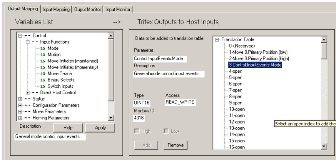
1. Select the *Input Mapping* tab (Input to the Tritex from the PLC)
