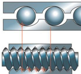
*Notice many more contact points on the roller screw compared to the ball screw. This results in higher load-carrying capacity and improved stiffness.*
