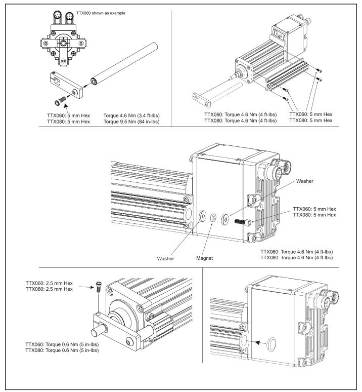
Figure 7 – Limit switch mounting
