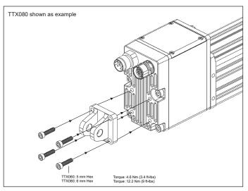
Figure 3 – Rear clevis mount (NOTE: Dimension drawings can be found in the Tritex TTX Series catalog or on the Exlar website.)
