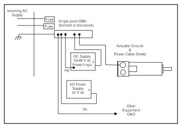
Figure 32 - Grounding Diagram
