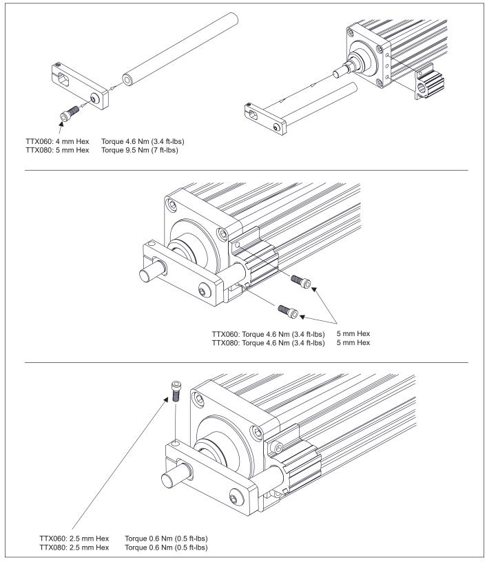
Figure 6 - Anti-rotation Assembly (shown in standard location)
