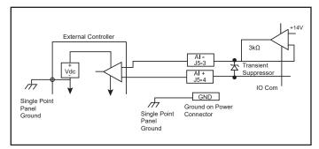
Figure 21 – Analog Output Wiring from External Controller
