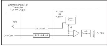
Figure 24 - Connection to High Side Controller
