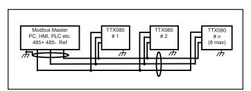
**Figure 23 –** Connecting multiple Tritex TTX actuators to a Modbus master Host
