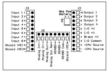
Figure 15 - Tritex TTX080 SIO and Ethernet Option
