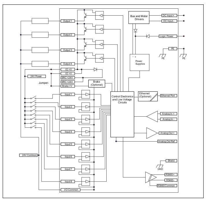
Figure 9 – Electrical Diagram STD I/O
