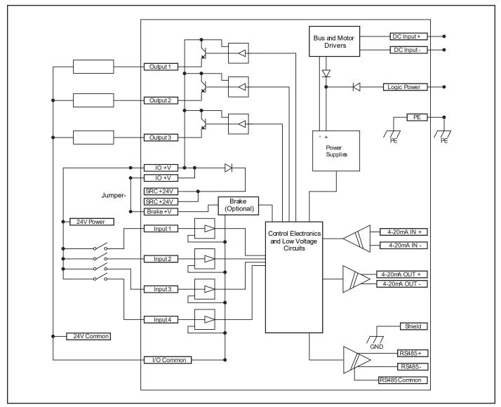
Figure 8 - Electrical Diagram 4-20 mA
