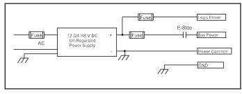
**Figure 29 –** Un-Regulated Power Supply for Logic and Bus Power
