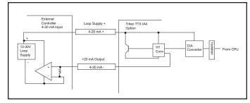
Figure 26 - 4-20 mA Output Connection
