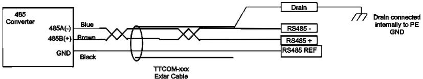
Typical RS485 connection to external converter
