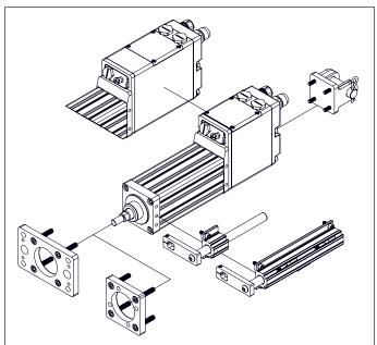
Figure 2 – Mounting configurations
