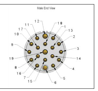
**Figure 23 –** Input /Output Standard M23 Connector Front View (19 pins)
