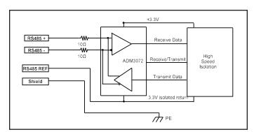
Figure 34 - Internal RS 485 Circuit
