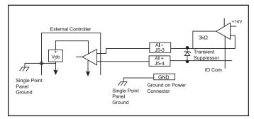
Figure 33 - Analog Output Wiring from External Controller
