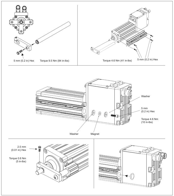
Figure 7 – Limit switch mounting
