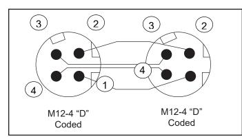
Figure 39 - M12 D Coded Straight Through Cord Set
