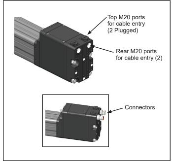
Figure 10 – M20 Cable Entry Ports
