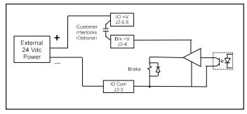
Figure 30 – Brake Connections with External 24V Power Supply
