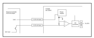
Figure 37 - Connection to Low Side Controller
