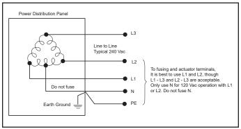
Figure 16 – Three Phase Delta with Mid-Phase GND Power Connection, 240 VAC
