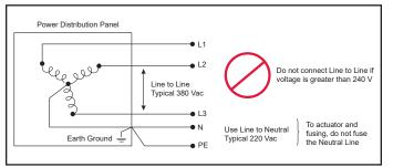
Figure 14 - Grounded WYE Power Connection, 220/380Y 3Φ
