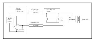
Figure 38 - 4-20mA Output Connection
