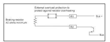
Figure 21 - Braking Resistor Connections
