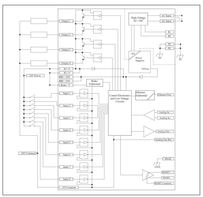
Figure 9 – Manual schematic STD I/O
