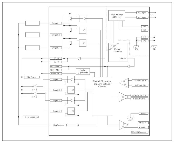
Figure 8 - Manual schematic 4-20 mA
