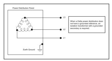
Figure 18 - Ungrounded Delta Power Distribution
