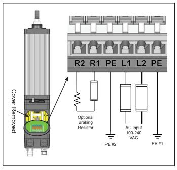
Figure 19 – Internal Power Terminal Block Connections
