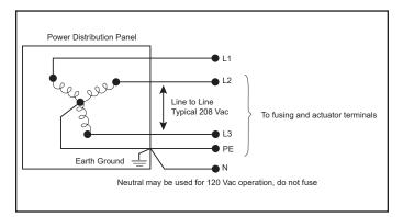
Figure 13 - Grounded WYE Power Connection, 120/208Y 3Φ
