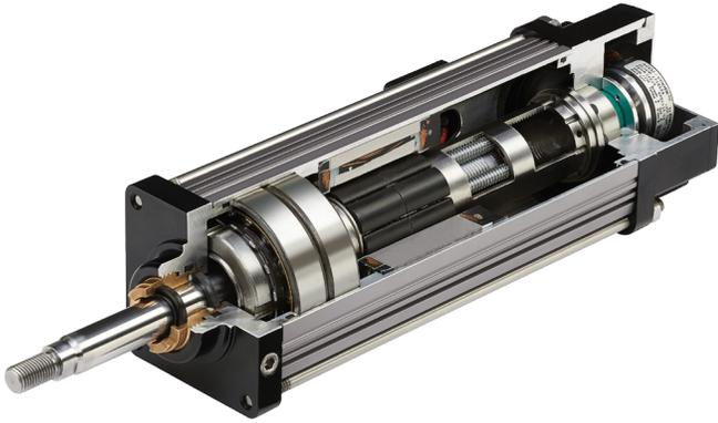
Electric actuators use roller screw technology, which enables high load capacity (more than 100,000 lb). Load capacity and rigidity of planetary roller screws suit applications requiring continuous force. Yet, these devices operate quietly, which helps in medical applications.
