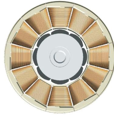
Figure 3: Minimized, non-overlapping end turns
