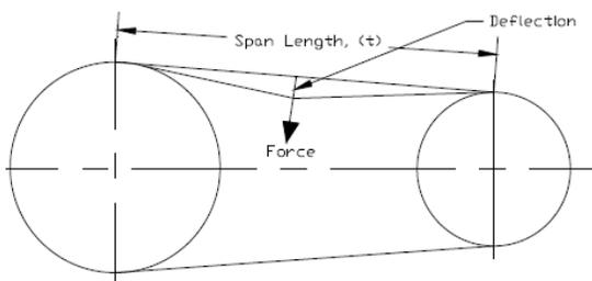
Figure 9: Belt Tension Diagram
