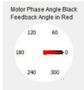
Note: Motor manufacturers typically align the resolver in 30 degree increments, typically by applying current through a pair of motor power wires.
