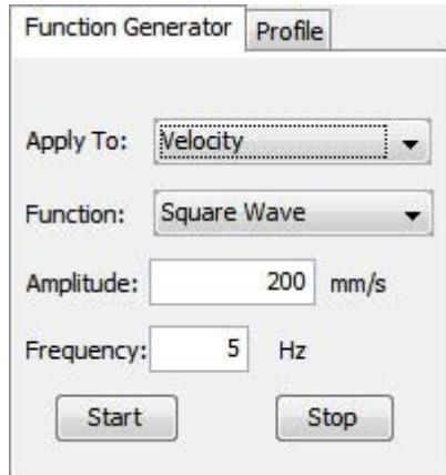
The **Start** button starts the function or profile generator. The **Stop** button stops the generator and aborts any profiles in progress.
