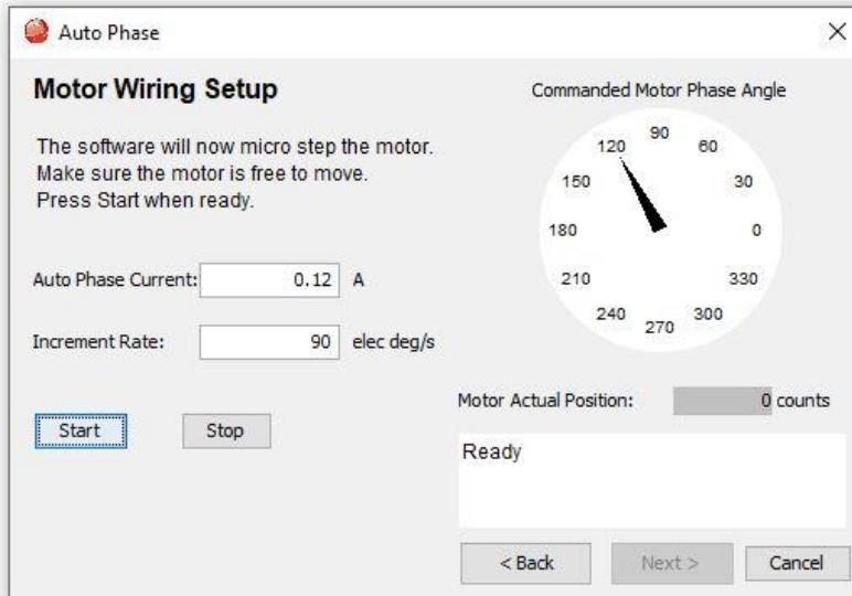
6. Click **Start** to begin the motor wiring setup.
