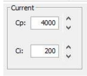
17. Adjust current loop integral gain (Ci) until desired settling time is obtained.
