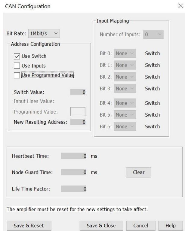
3. Choose a Bit Rate and choose any combination of address sources (Switch, Inputs, and Programmed Value). The address is the sum of the values from these sources.
