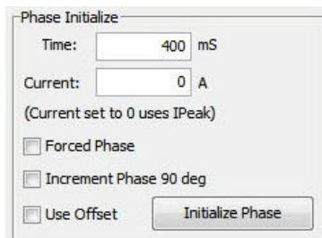
If the phasing function fails (for instance, message "Phase Initialized" is not displayed, or if a phasing fault is indicated) adjust the phase initialization settings described below and try Step 4 (**Initialize Phase**) again.
