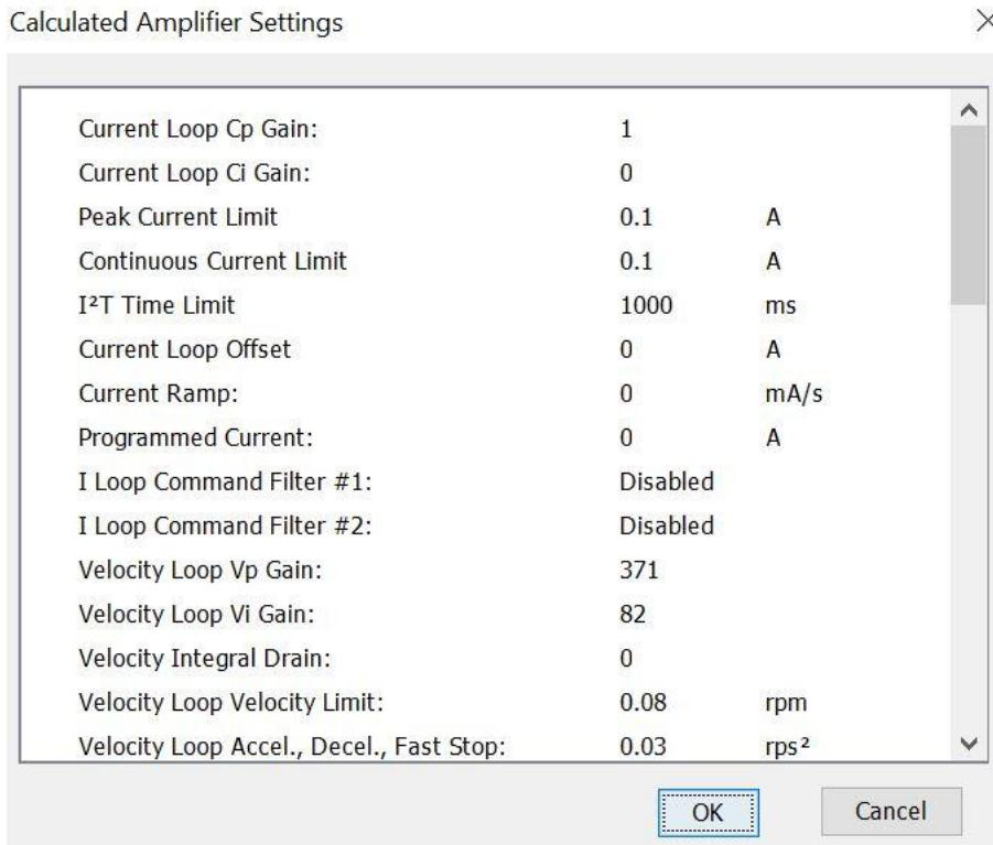
2. Verify the peak current limit, continuous current limit, and velocity loop velocity limit. If one or more of these values seems inappropriate, click **Cancel** and check: Peak Torque (or Force), Continuous Torque (or Force), Velocity Limit, and Torque (or Force) Constant. Correct them if needed. See Rotary Motor Parameters or **Error! Reference source not found.**
