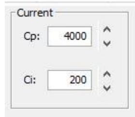
7. Adjust current loop integral gain (Ci) until desired settling time is obtained.
