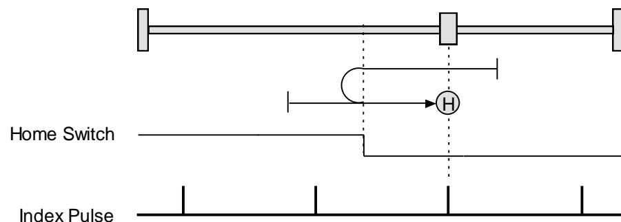
**Home Switch In to Index****Direction of Motion: Positive**
