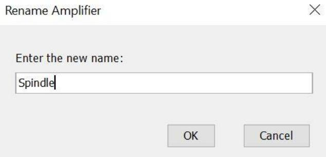
3. Enter the new name and click **OK** to close the screen. The Drive name is now in FLASH and can be seen in the tree.
