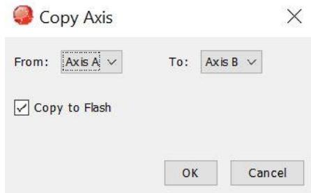
Select the source and destination axes, then click **OK**. Note that Copy to Flash is selected by default. If this option is not selected, then the RAM/Flash parameters will only be copied to the destination axis' RAM, while still copying the Flash Only data to the destination axis' Flash.
