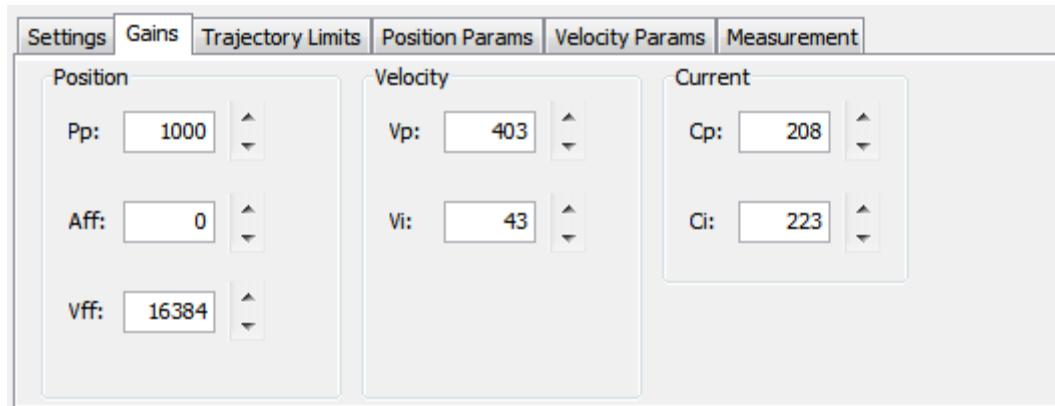
Note that the parameters represented on these tabs can also be accessed through the screens used to configure the control loops and the digital position input. Changing a value in the Scope tool automatically updates the value on the other screens where it appears, and vice versa.
