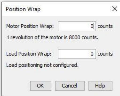
Change/verify the position wrap parameters as needed. Set both values to zero to disable position wrapping. Note that the changes do not take effect until **OK** is pressed. For more information about this feature, see Position Wrap.
