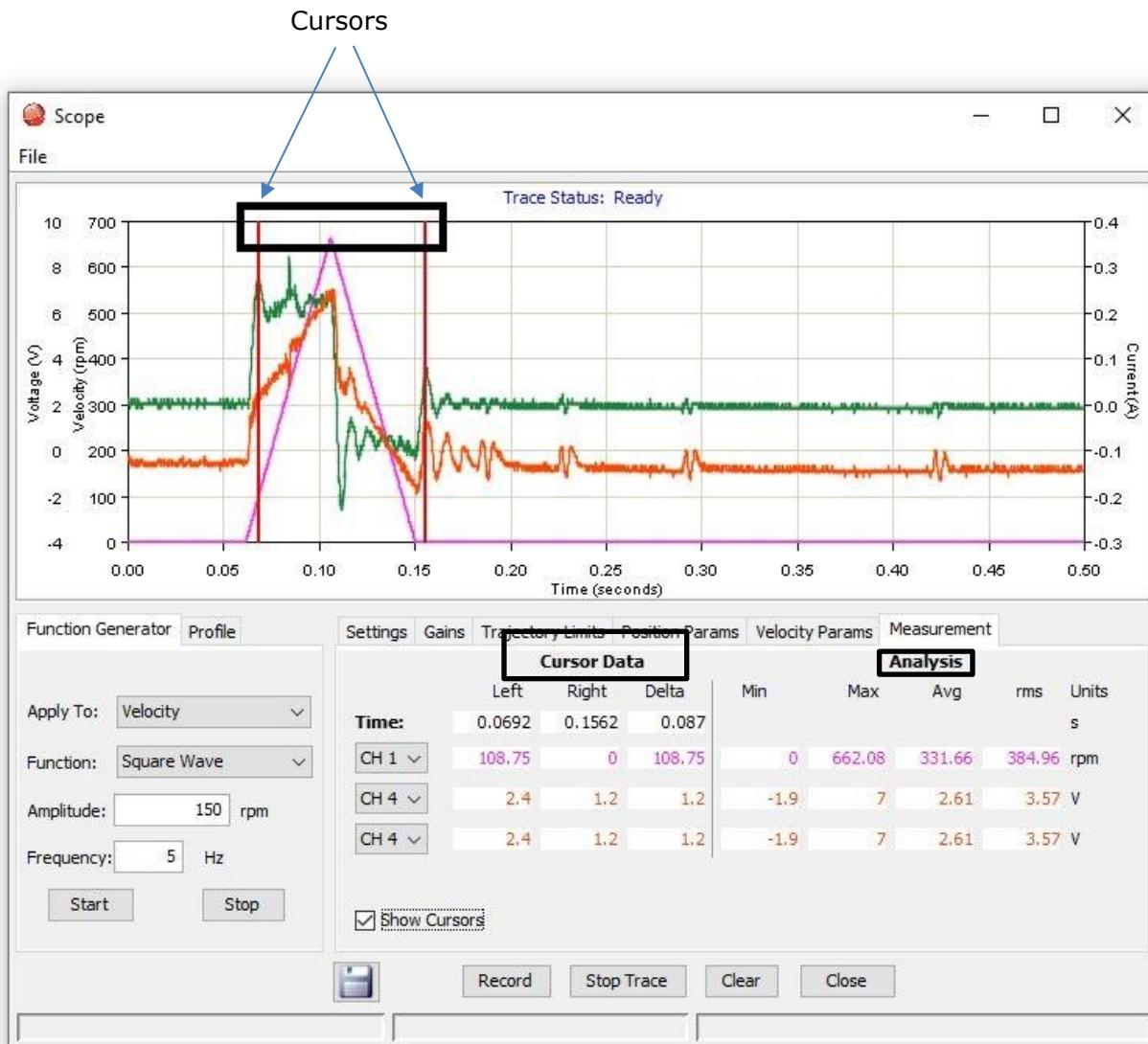
When **Show Cursors** is not set, the Cursor Data fields are inactive and the Analysis fields show calculations based on data from the entire trace cycle.
