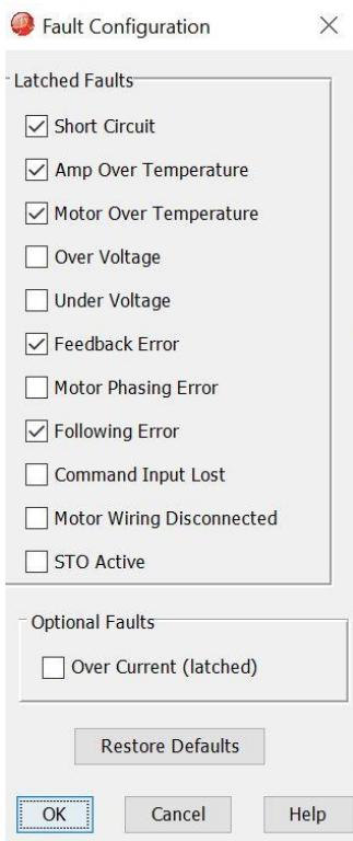
2. Select the faults to latch. See Fault Descriptions.
