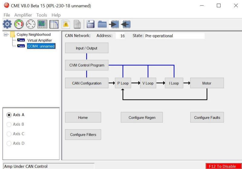
Example of a CME Main Screen after an amplifier has been selected.
