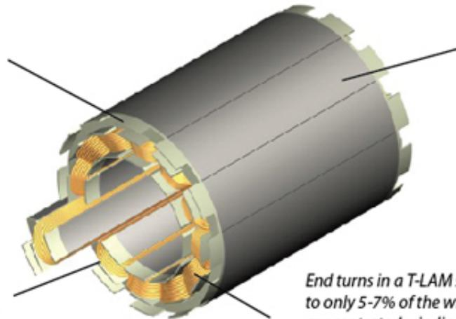
Wound segments are combined and held together to complete the stator sub-assembly.
