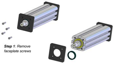
**Step 2**: Remove faceplate and rod wiper. If O-Ring does not stay in place, remove that as well (IP65 units only)
