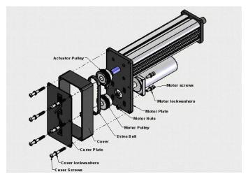
Figure 9: Parallel Motor Mount Drive Train Assembly
