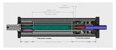
Figure 10-1: Actuator Shown in fully retracted "crash" position, with contact on forward impact bumper
