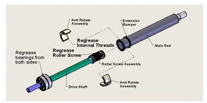
Figure 14: Actuator Disassembly
