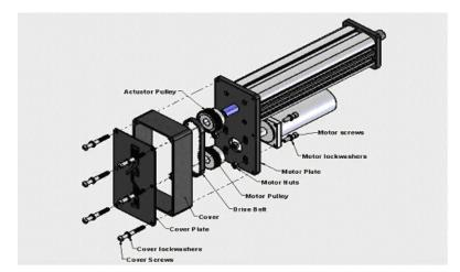
Figure 11: Parallel Motor Mount Drive Train Assembly
