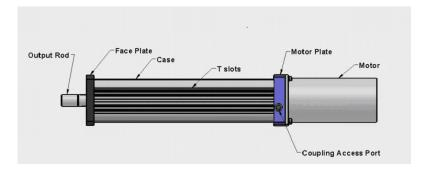
Figure 4: I Series with Inline Motor Mount
