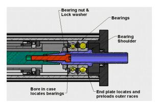
Figure 8: Roller Screw Support Bearing Detail
