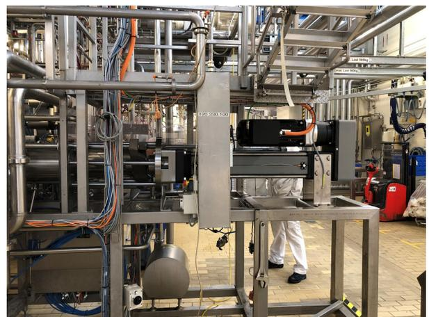
Using only the data provided from the previous hydraulic system, a new electrical system was designed for Mittelland Molkerei AG; by analyzing how often the system would need above-average force they were able to design a system that was perfectly sufficient to handle normal production without being overbuilt.
