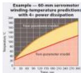
Furthermore, thermodynamics teaches that for heat to flow from within the motor out towards its exposed surface area, there must be a temperature gradient both within the motor and between the motor and the ambient environment. Depending on motor size and operating temperature there can be as much as a 30 to 50 $^{\circ}\text{C}$  temperature difference between the electrical winding and its exposed outermost surface area. This difference can't be ignored.
