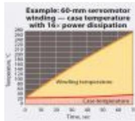
It is evident from the graphs that the two-parameter model becomes inaccurate once the power dissipation exceeds the 1× maximum continuous value. The temperature difference between what the two thermal models predict grows progressively worse with rising power dissipation. To verify this last statement, compare
