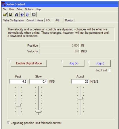
Jog Slow: The Jog speed when the Fast Jog is not selected Jog Fast: The Jog speed when the Fast Jog is selected Jog Acceleration: The Acceleration and Deceleration ramp used in Jog Mode
