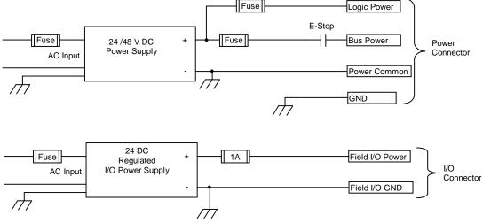
2 power supply configuration, maintaining I/O Isolation
