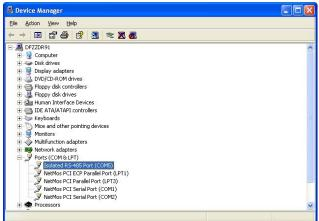
The Name of the device driver that has been installed must show under Ports, if it does not the Expert Software cannot connect to the PC COM port. Notice the COM#, COM5 in the example above; use this COM port number in the Expert Softer when setting up PC communication. Double Click on the COM Port to see the screen below to verify the converter's device driver is working.
