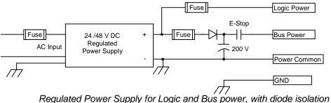
ated Power Supply for Logic and Bus power, with diode is and optional extra capacitance
