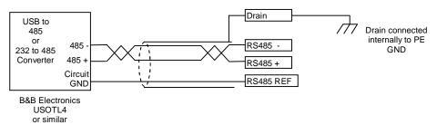
Typical RS 485 connection to external converter
