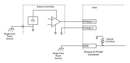
Analog input wiring from voltage or current control external controller
