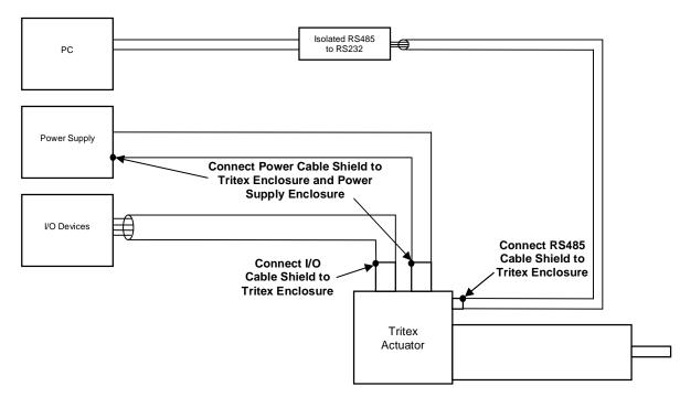
Cable Shield Grounding Example
