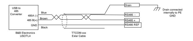
Connection to B&B USOTL4 using TTCOM cable
