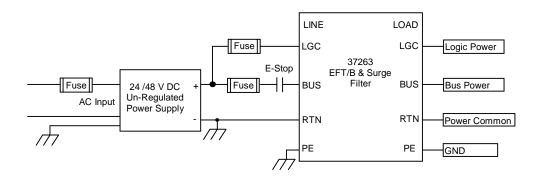
Power Connection using External EFT/B & Surge Filter
