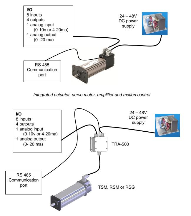
Integrated actuator and servo motor with remote drive amplifier and motion control
