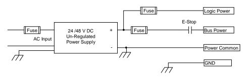
Un-Regulated Power Supply for Logic and Bus power
