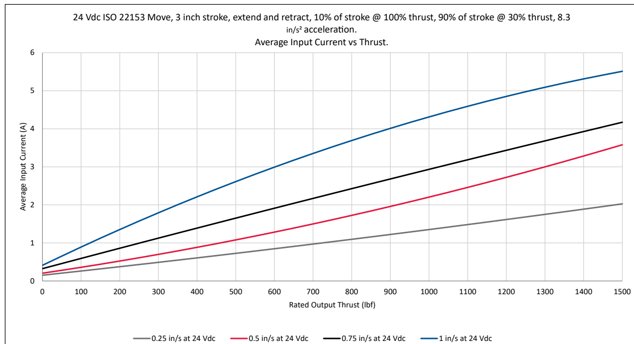
Figure 5 - 24 Vdc Average Input Current vs Thrust
