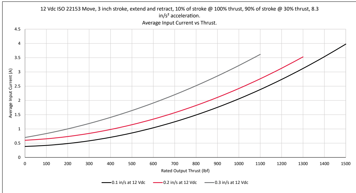
Figure 4 - 12 Vdc Average Input Current vs Thrust
