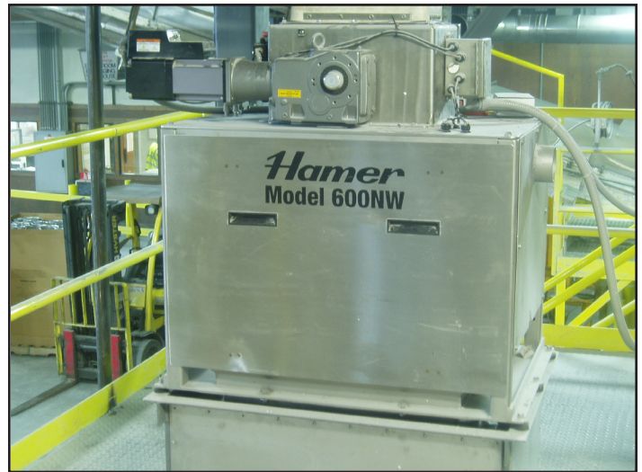
Hamer's Model 600NW Net Weigh Scale with Exlar's Tritex II AC rotary actuator.
