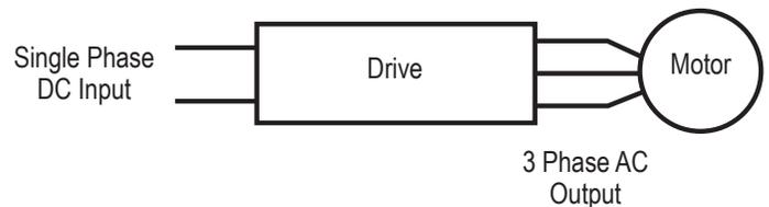
$$\text{Input Watts} = \text{input Volts (dc)} \times \text{Input Amps (dc)}$$
