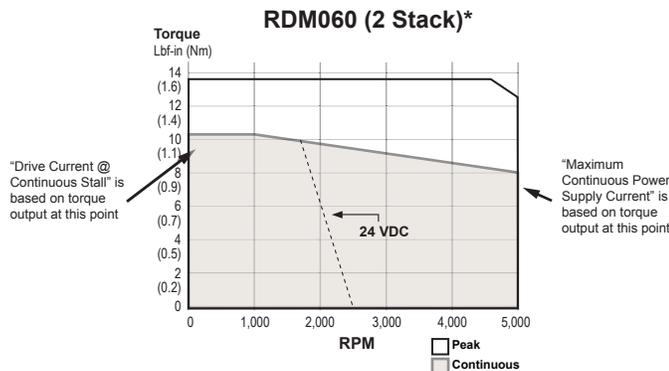
\*Using NEMA recommended aluminum heatsink 10 X 10 X 1/4 inch
